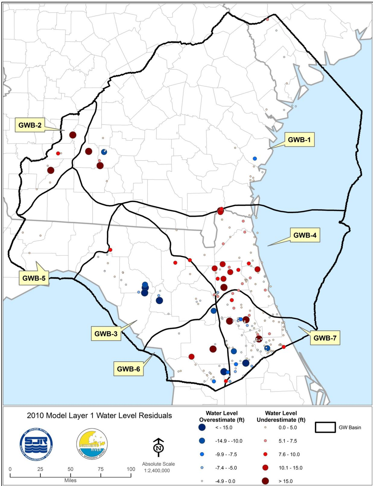
Figure 5-21. 2010 groundwater level residuals, model Layer 1
