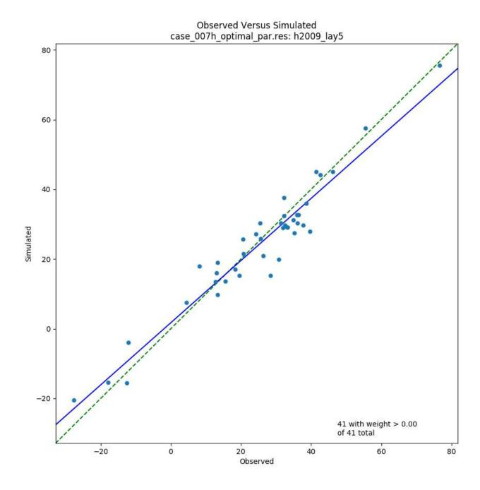
Figure 4-38. Observed versus simulated hydraulic head (feet NAVD88), model Layer 5, 2009
