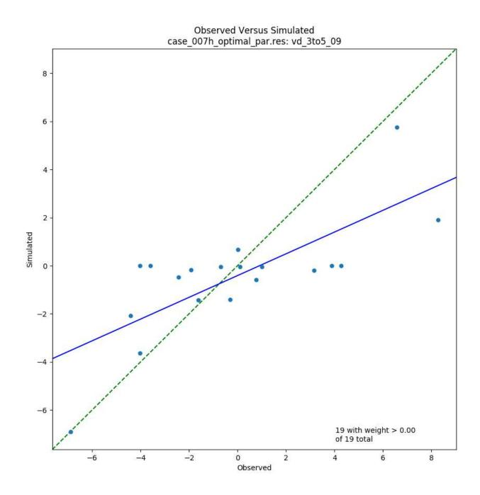
Figure 4-34. Observed versus simulated vertical head differences (feet), model Layers 3 and 5, 2009
