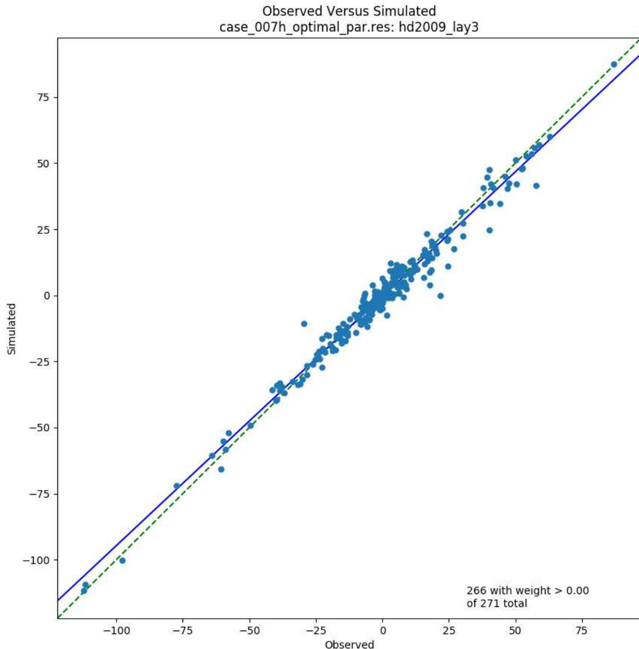
Figure 4-28. Observed versus simulated horizontal head differences (feet), model Layer 3, 2009
