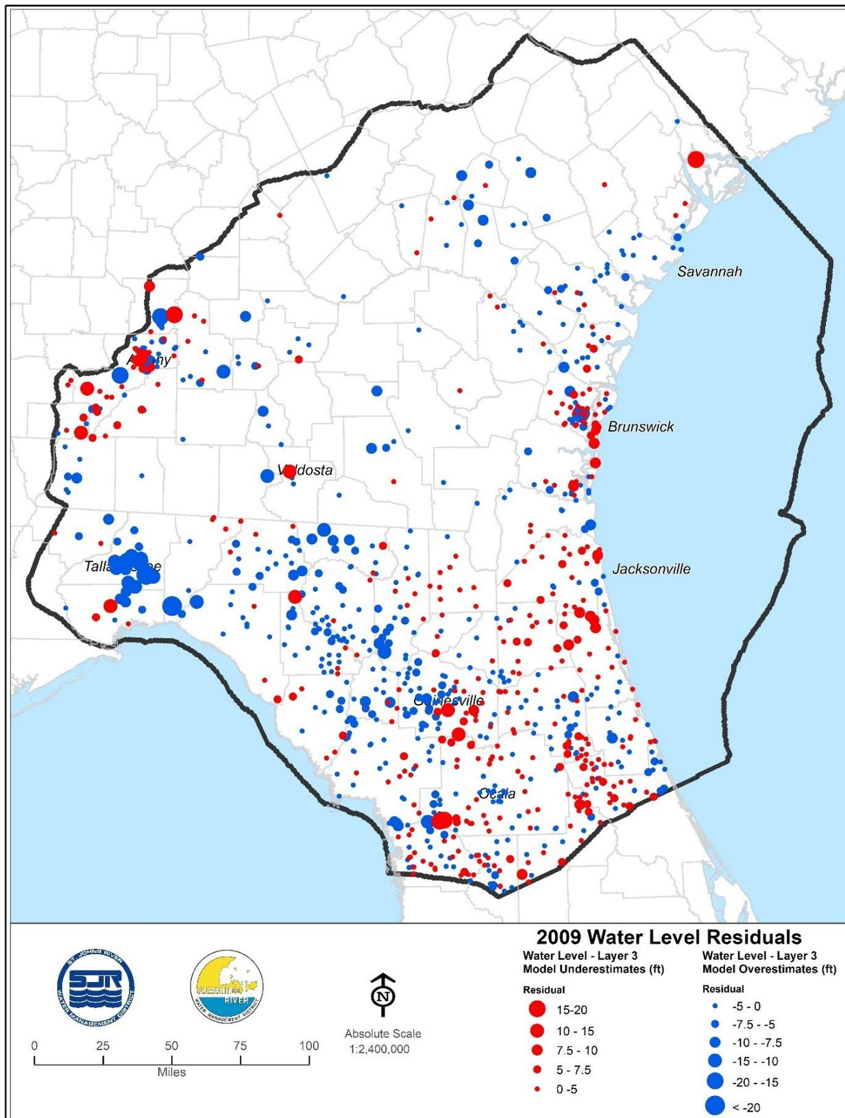
Figure 4-22 (a). Residuals of Hydraulic Head (Feet), Model Layer 3, 2009
