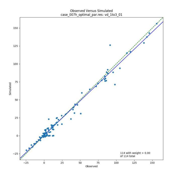
Figure 4-19. Observed versus simulated vertical head differences (feet), model Layers 1 and 3, 2001
