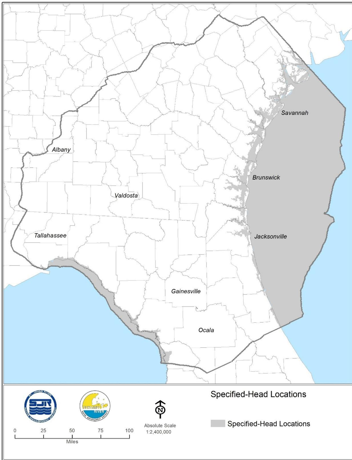
Figure 3-45. Distribution of specified-head grid cells in Layer 1
