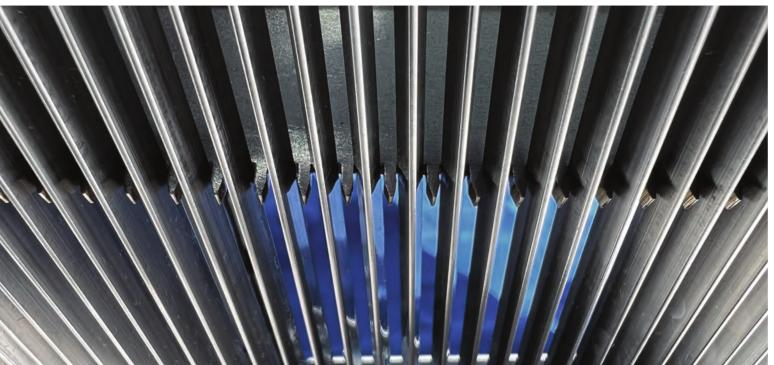
Precisely engineered rakes clean the bar array to ensure clog free operation without washwater or brushes.
