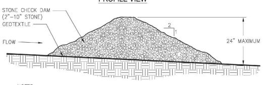
CHECK DAMS ARE TO BE USED ONLY IN SMALL OPEN CHANNELS (THEY ARE NOT TO THE DRAINAGE AREA FOR STONE CHECK DAMS SHALL NOT EXCEED TWO ACRES.
