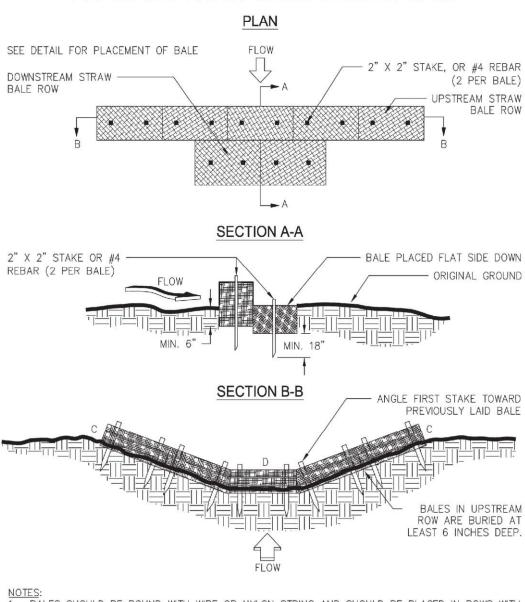
1. BALES SHOULD BE BOUND WITH WIRE OR NYLON STRING AND SHOULD BE PLACED IN ROWS WITH BALE ENDS <u>TIGHTLY</u> ABUTTING THE ADJACENT BALES.
