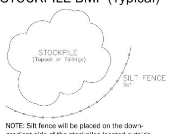
gradient side of the stockpiles located outside of the PCP/WCP area.
