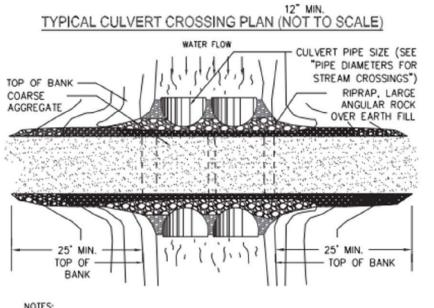
HIS TYPE OF CROSSING CAN BE INSTALLED IN BOTH A WET OR DRY WEATHER STREAM CONDITION WHERE THE DRAINAGE AREA EXCEEDS 10 ACRES 2. REMOVE DURING CLEANUP.
