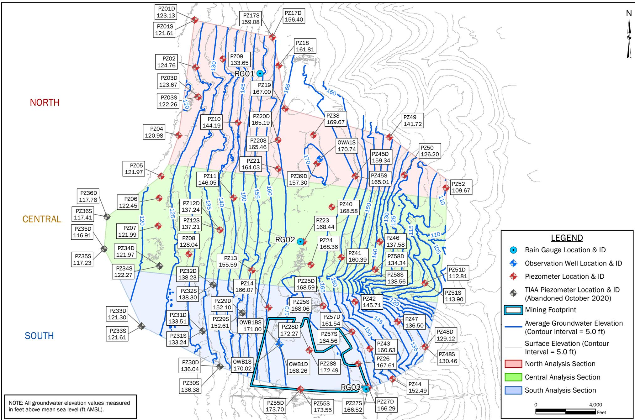
**FIGURE 2: MEAN GROUNDWATER ELEVATIONS, OBSERVATION WELL & PIEZOMETER LOCATIONS & ANALYZED SECTIONS MAP**
