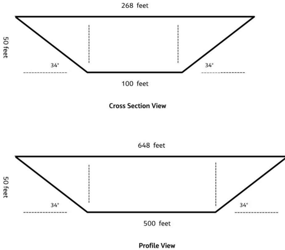
Figure 2. Mine Pit Conceptual Model (X-section and Profile)
