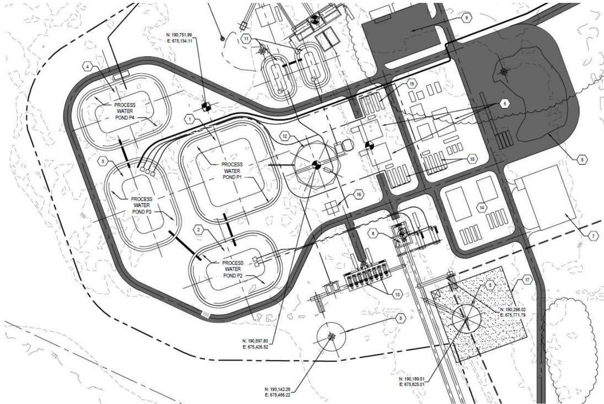
The Process Water Ponds (P1–P4) will be above-ground and lined. Lining details for all ponds are shown on Sheet C-701. The individual pond volumes are shown on Sheet C-200; as shown in the table below, the total capacity of the four ponds is approximately 3.9 MG, and the working capacity with appropriate freeboard is 3.4 MG.
