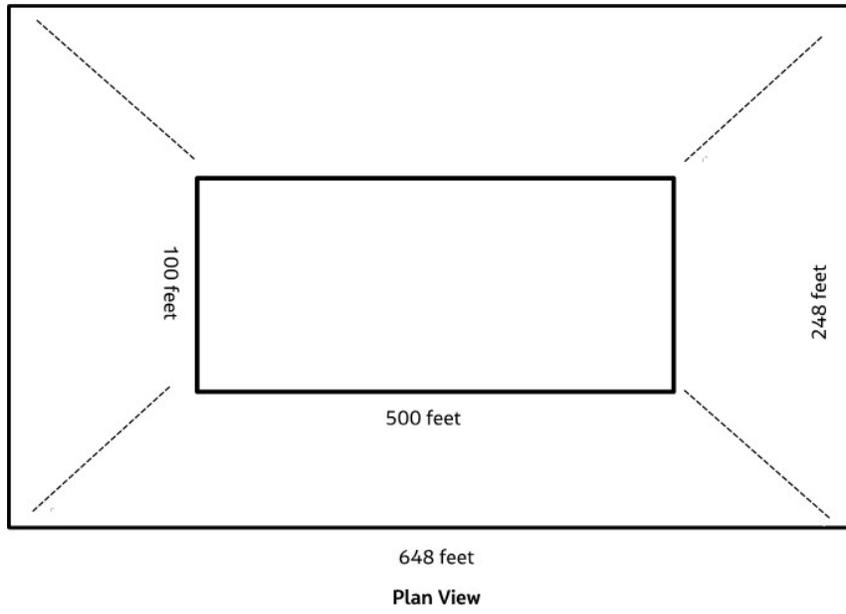
Figure 1. Mine Pit Conceptual Model
