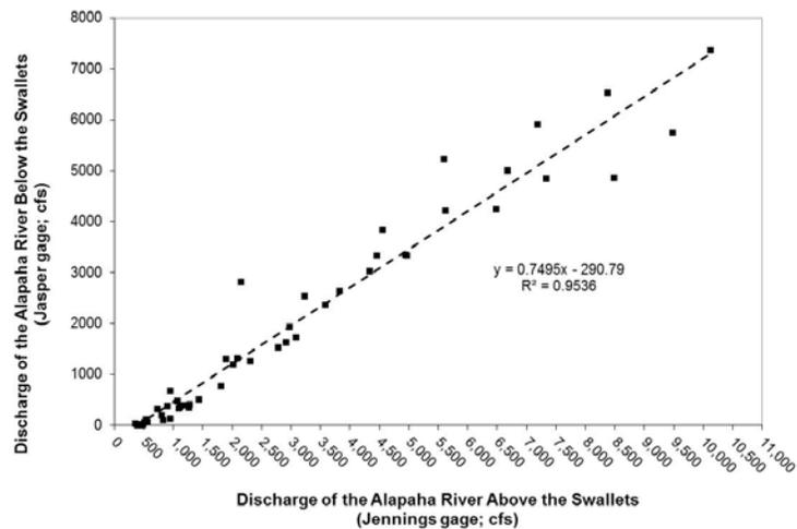
**Figure 21. Comparison of the measured discharge of the Alapaha River at Jasper with measured or modeled discharge at the Jennings gages.**
