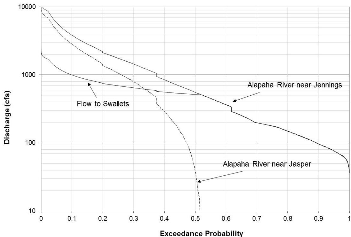
**Figure 28. Flow-duration curves for the Alapaha River above and below the swallets and, by difference, flow into the swallet system.**
