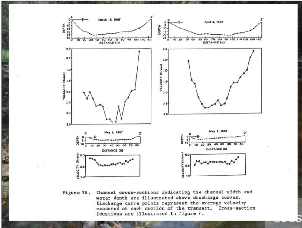
Figure 38. Channel cross-sections indicating the channel width and water depth are illustrated above discharge curves. Discharge curve points represent the average velocity measured at each section of the transect. Cross-section locations are illustrated in figure 7.
