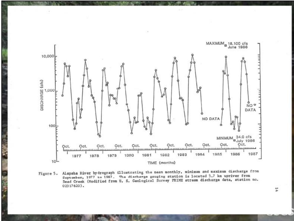
Figure 5. Alapaha River hydrograph illustrating the mean monthly, minimum and maximum discharge from September, 1977 to 1987. The discharge gauging station is located 3.7 km upriver from Dead Creek (Modified from U. S. Geological Survey PRIME stream discharge data, station no. 02317620).
