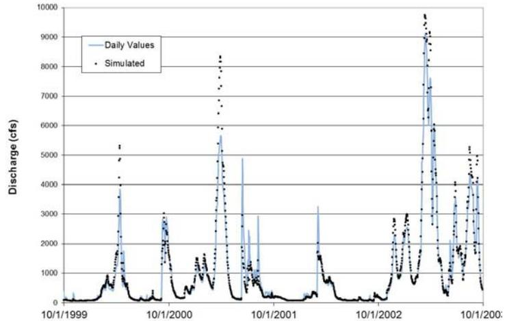
**Figure 20. Comparison of modeled and measured discharge of the Alapaha River at the Jennings gage.**
