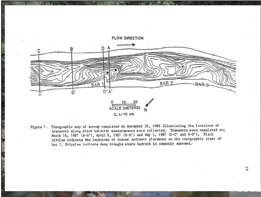
Figure 7. Topographic map of survey completed on November 23, 1986 illustrating the locations of transects along which velocity measurements were collected. Transects were completed on; March 16, 1987 (A-A'), April 6, 1987 (B-B') and May 1, 1987 (C-C' and D-D'). Black circles indicate the locations of tracer sediment placement on the topographic crest of bar 1. Stipples indicate deep troughs where bedrock is commonly exposed.
