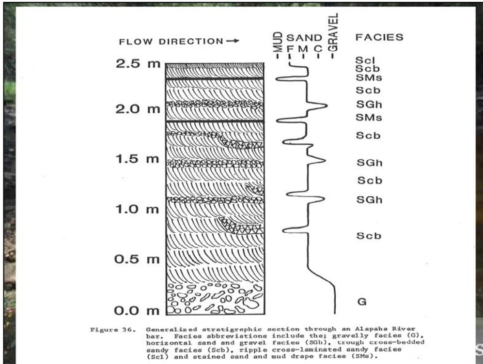
After determining facies, I described them in cross-section, so you could essentially determine depositional environment with a core. I defined facies called gravelly facies (G), horizontal sand and gravel facies (SGh), trough cross-bedded sandy facies (Scb), ripple cross-laminated sandy facies (Scl) and stained sand and mud drape facies (SMs).
