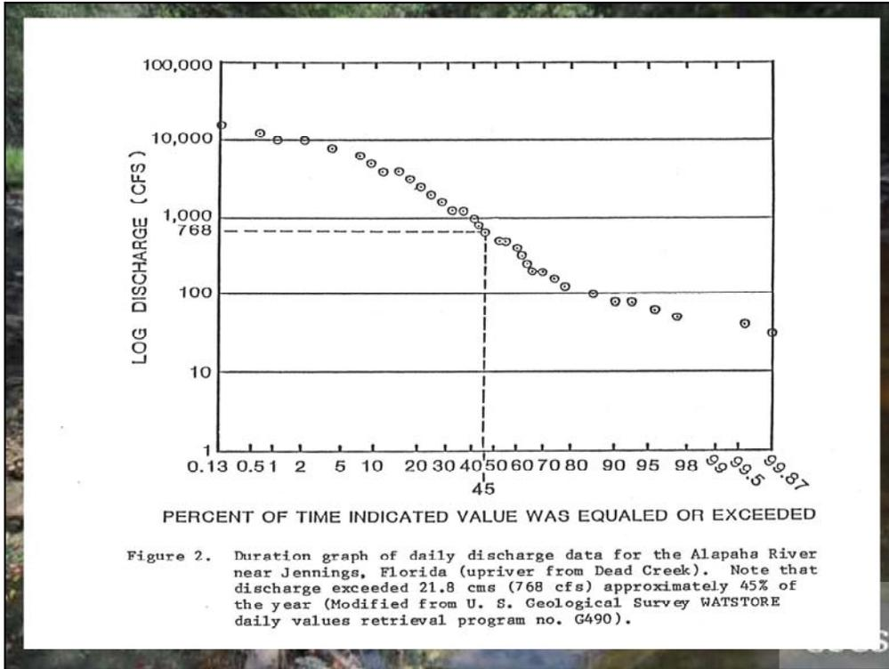
Of course my thesis was heavy on data evaluation. This graph indicates that the Alapaha river discharge exceeded the volume that flows into the ground at Dead River 45% of the time.
