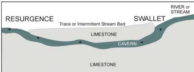
**Figure 7a – Cross section of a swallet-resurgence system.**
