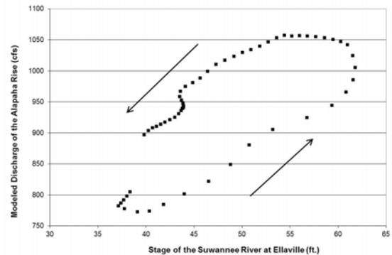
**Figure 27. Hysteresis loop at the Alapaha Rise for the Suwannee River flood of February 11 through March 31, 1986.**
