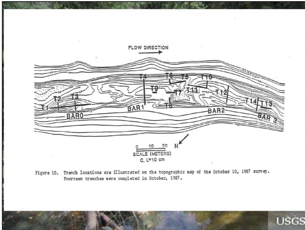
Figure 10. Trench locations are illustrated on the topographic map of the October 10, 1987 survey. Fourteen trenches were completed in October, 1987.
