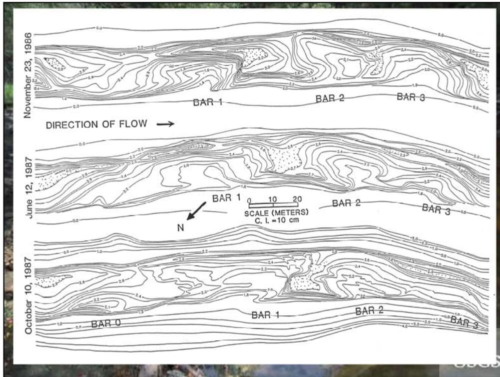
I made topo maps of the meander at different times to document that this environment is very much non-static. This is primarily due to the fact that the sediment exists within a limestone channel, as opposed to a completely unconsolidated environment.
