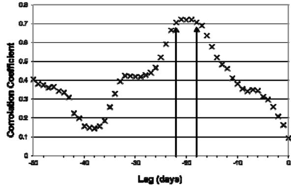
Figure 24. Cross-correlation analysis of lag time between discharge at the Jennings gage on the Alapaha River with discharge at the Alapaha Rise when discharge at Jennings is > 500 cfs. The peak discharge ranges from 18 to 21 days.
