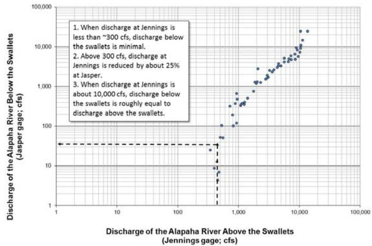
**Figure 22. Comparison of discharge above and below the swallet system using modeled data.**
