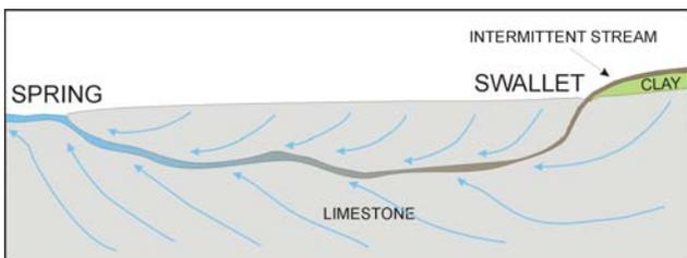
**Figure 7b – Cross section of a swallet-to-spring system fed by an intermittent stream.**
