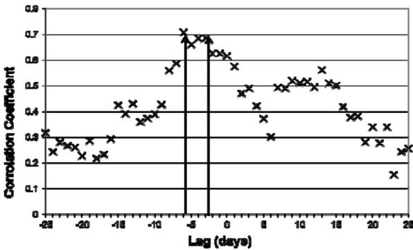
Figure 23. Cross-correlation analysis of lag time between discharge at the Jennings gage on the Alapaha River with discharge at the Alapaha Rise when discharge at Jennings is < 500 cfs. The peak discharge ranges from 3 to 6 days.
