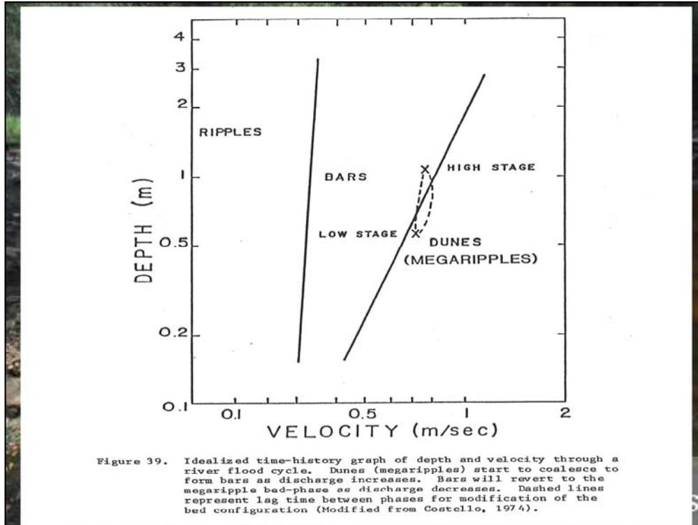
Figure 39. Idealized time-history graph of depth and velocity through a river flood cycle. Dunes (megaripples) start to coalesce to form bars as discharge increases. Bars will revert to the megaripple bed-phase as discharge decreases. Dashed lines represent lag time between phases for modification of the bed configuration (Modified from Costello, 1974).
