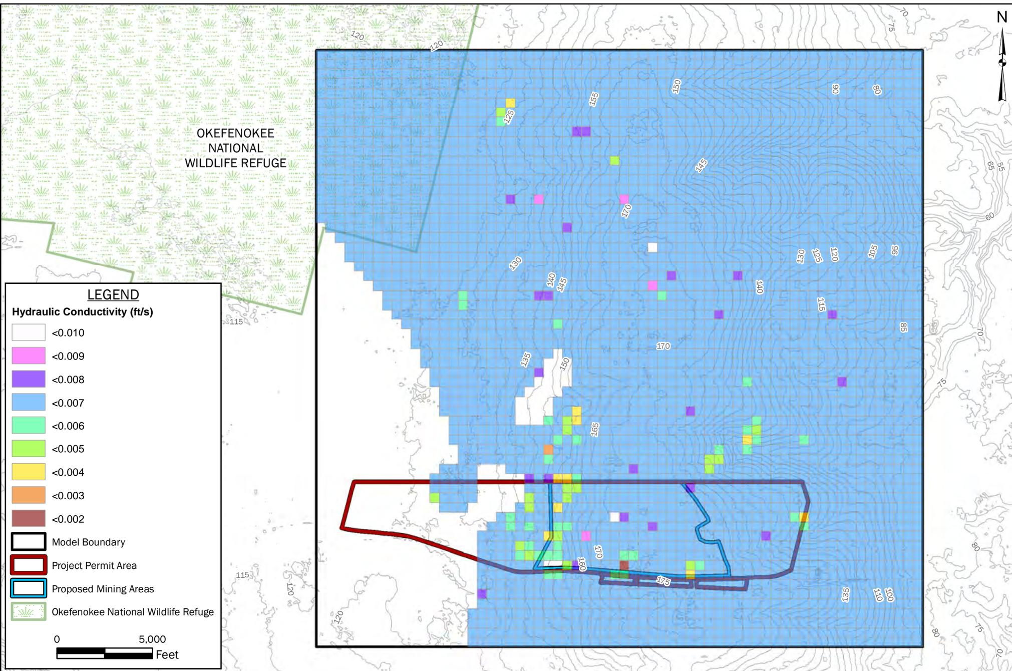
**FIGURE 25: INITIAL MODEL HORIZONTAL HYDRAULIC CONDUCTIVITY LAYER 11**
