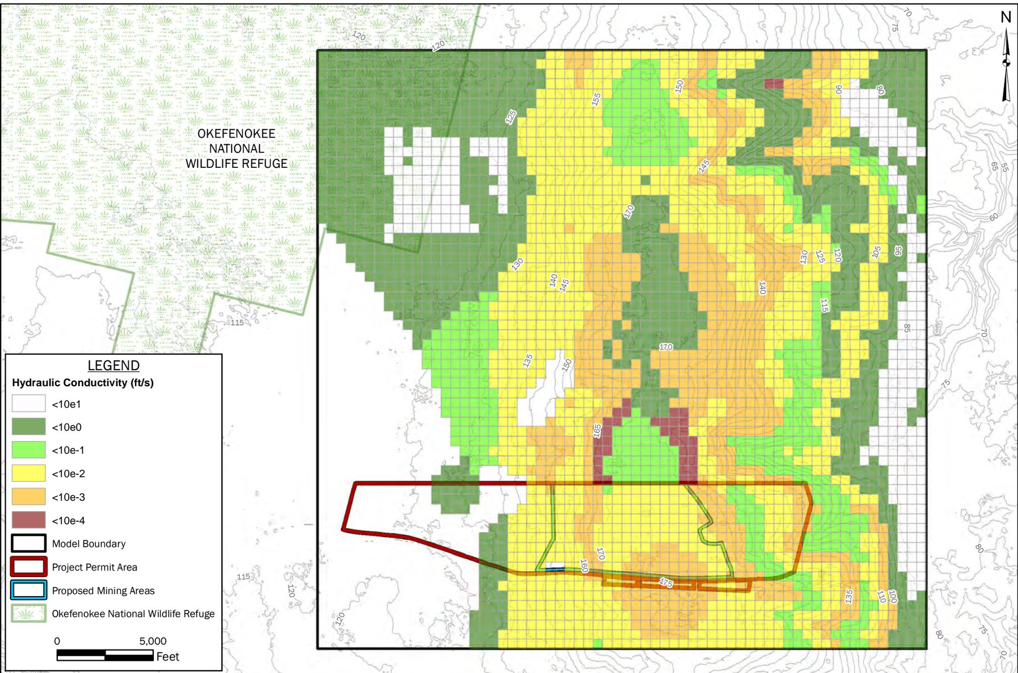
**FIGURE 42: CALIBRATED MODEL HORIZONTAL HYDRAULIC CONDUCTIVITY LAYER 11**
