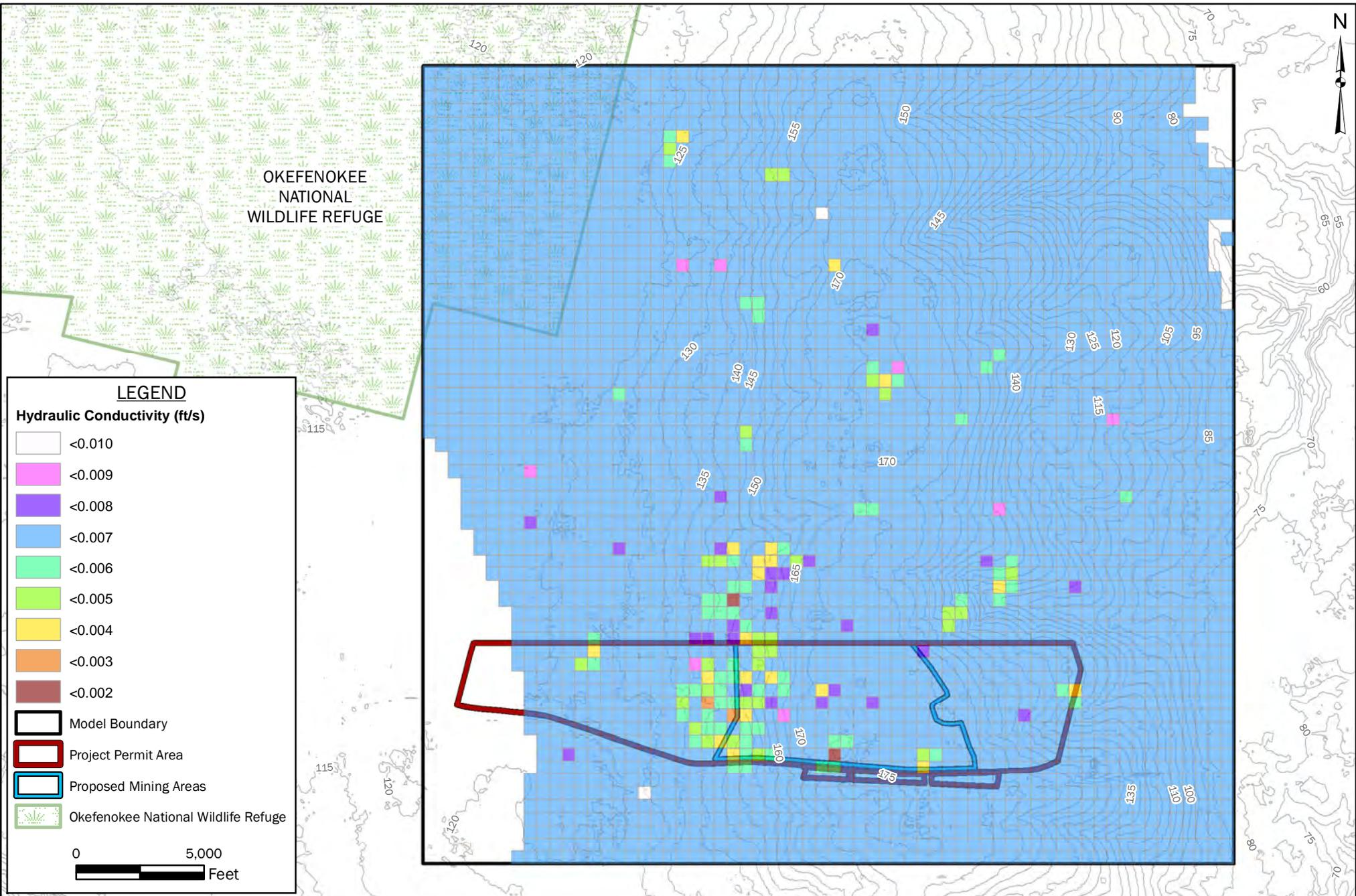
**FIGURE 24: INITIAL MODEL HORIZONTAL HYDRAULIC CONDUCTIVITY LAYER 10**
