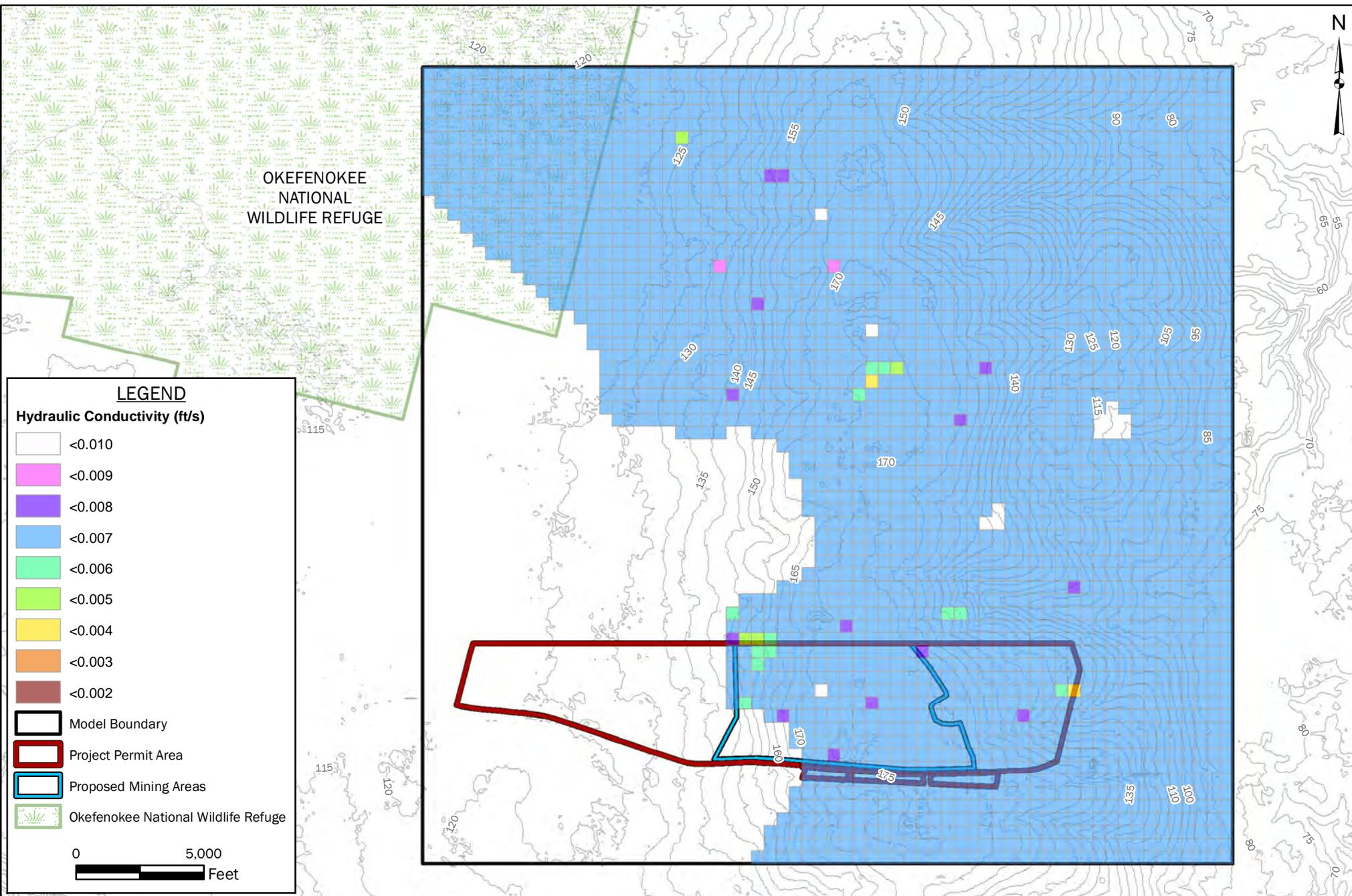
FIGURE 26: INITIAL MODEL HORIZONTAL HYDRAULIC CONDUCTIVITY LAYER 12
