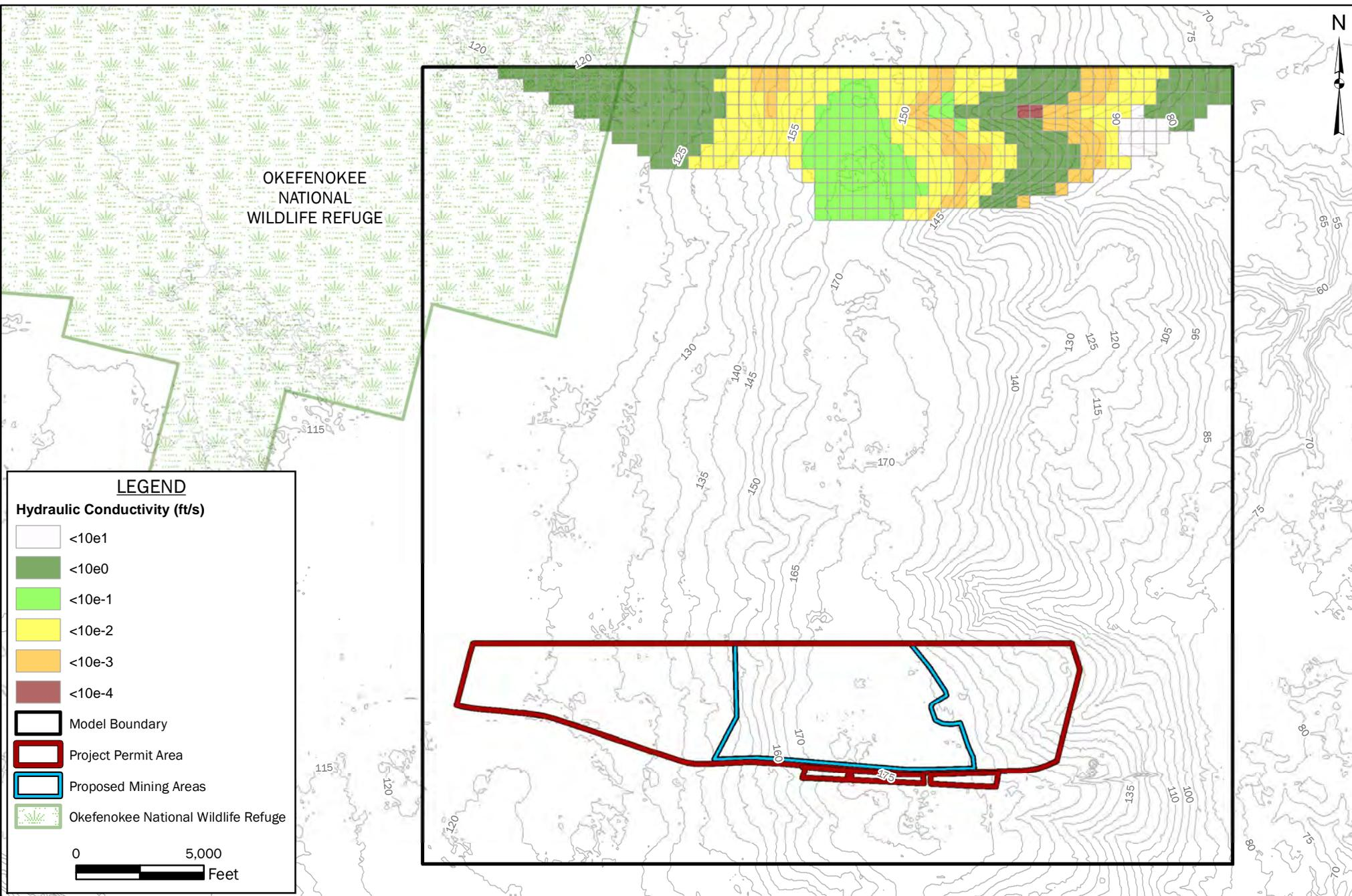
**FIGURE 45: CALIBRATED MODEL HORIZONTAL HYDRAULIC CONDUCTIVITY LAYER 14**
