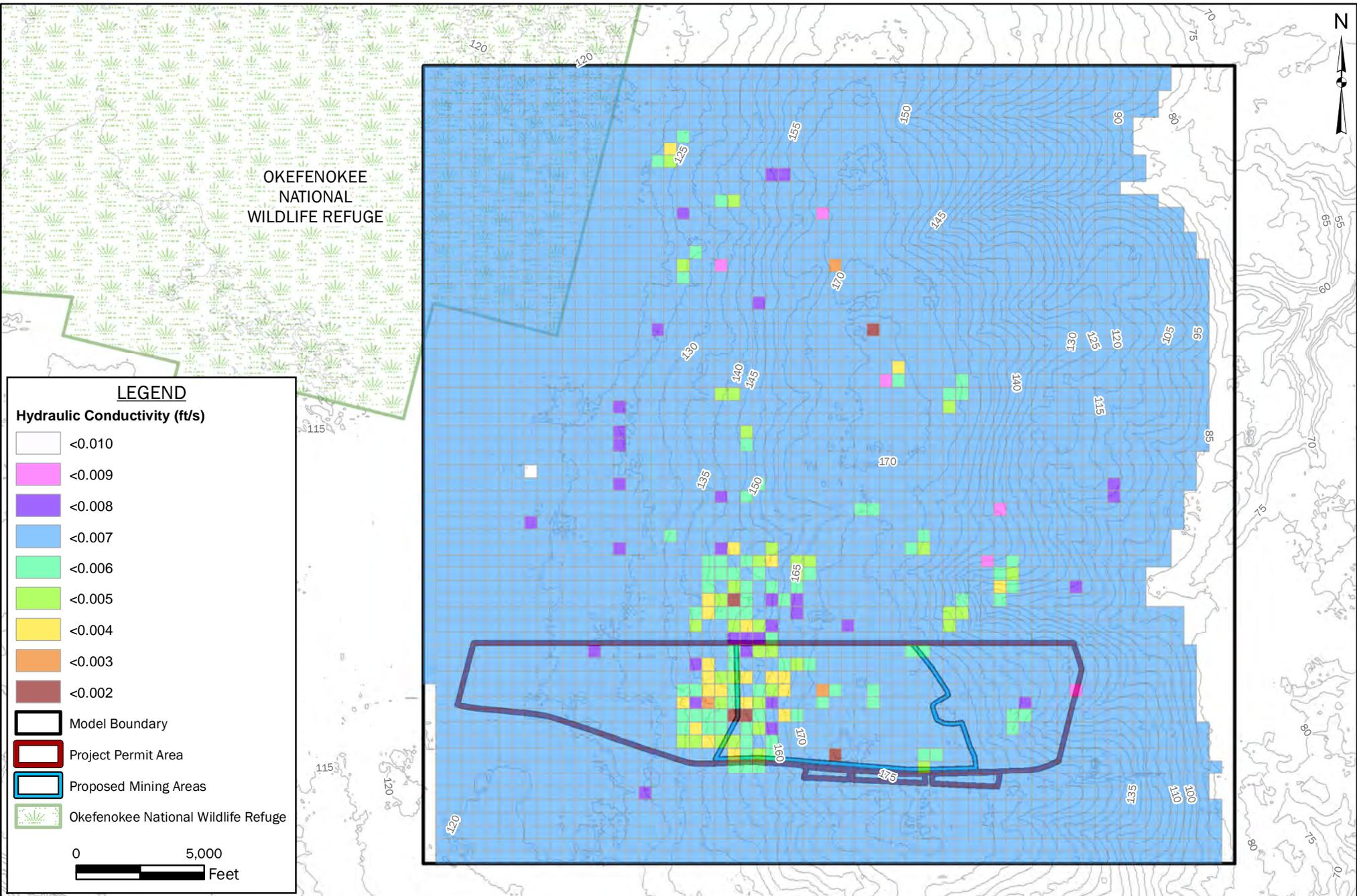
**FIGURE 23: INITIAL MODEL HORIZONTAL HYDRAULIC CONDUCTIVITY LAYER 9**
