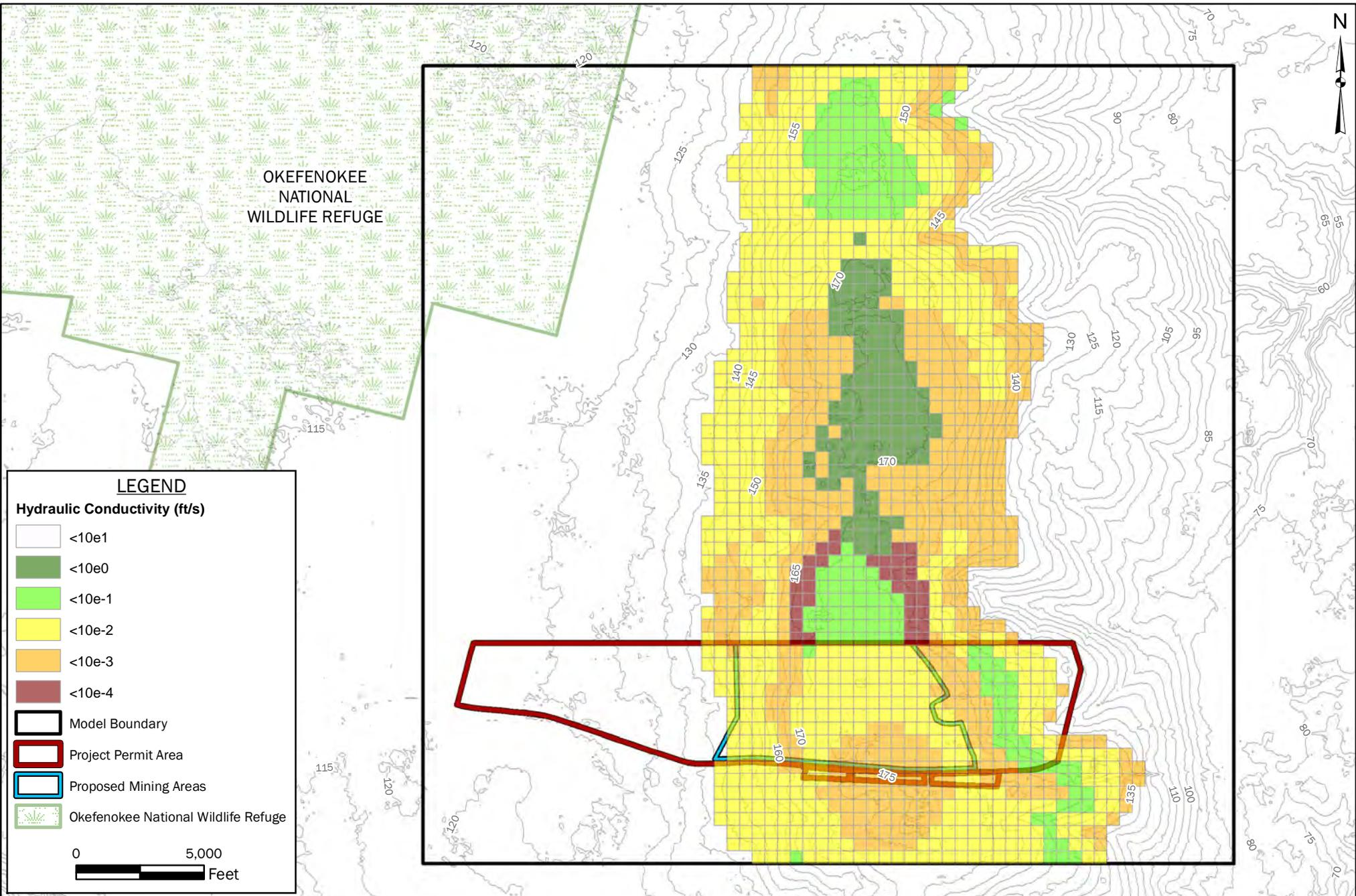
**FIGURE 35: CALIBRATED MODEL HORIZONTAL HYDRAULIC CONDUCTIVITY LAYER 4**
