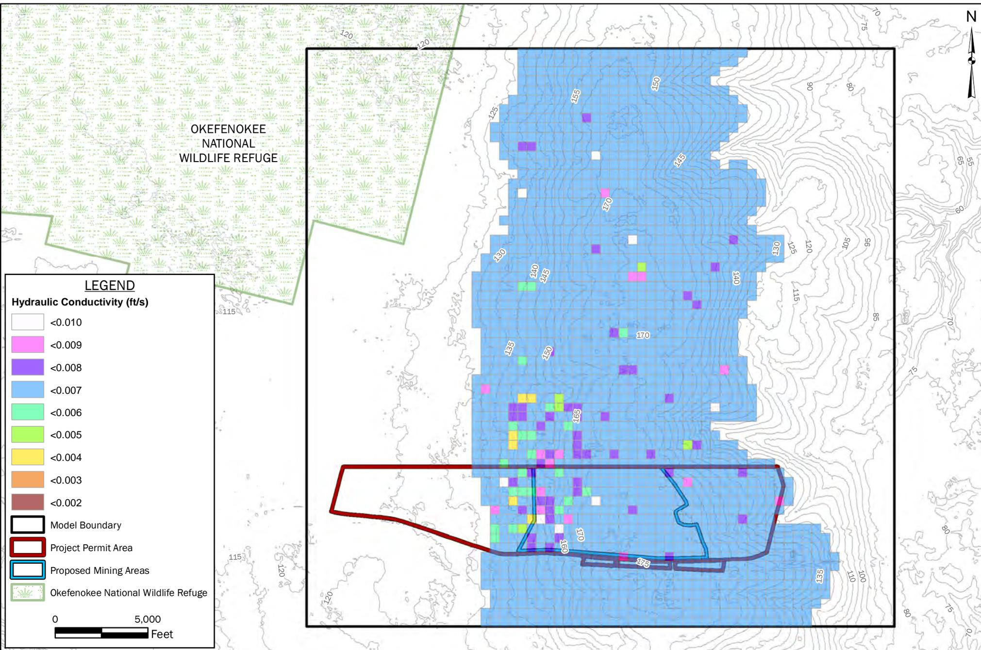
**FIGURE 19: INITIAL MODEL HORIZONTAL HYDRAULIC CONDUCTIVITY LAYER 5**
