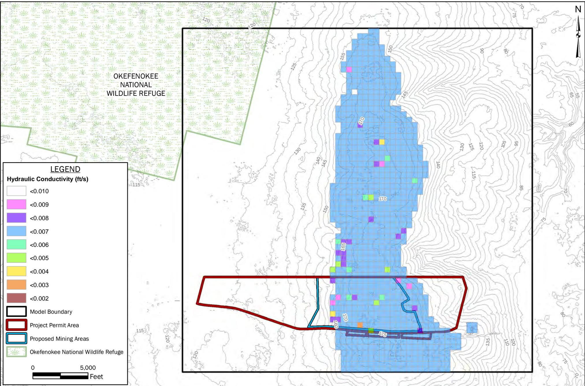
**FIGURE 16: INITIAL MODEL HORIZONTAL HYDRAULIC CONDUCTIVITY LAYER 2**
