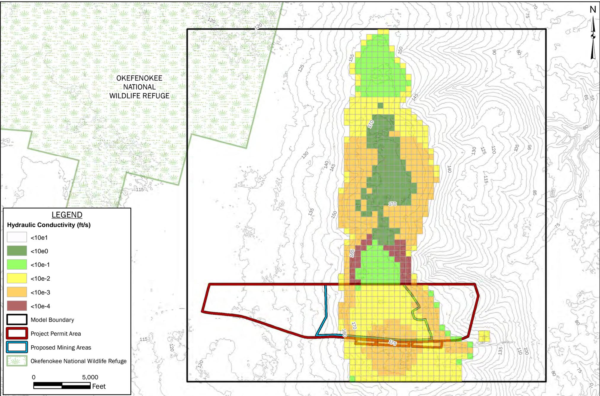
**FIGURE 33: CALIBRATED MODEL HORIZONTAL HYDRAULIC CONDUCTIVITY LAYER 2**
