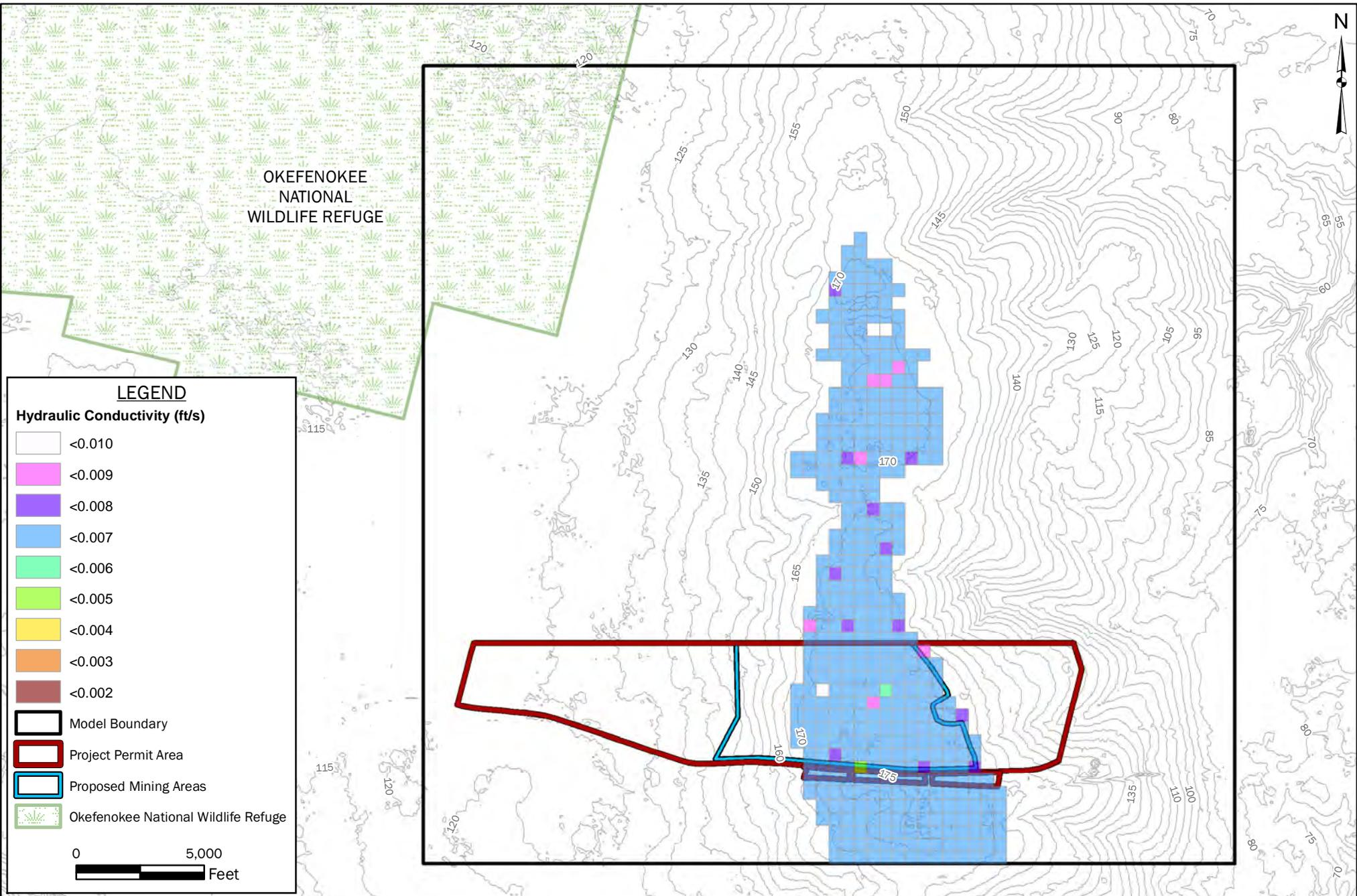
**FIGURE 15: INITIAL MODEL HORIZONTAL HYDRAULIC CONDUCTIVITY LAYER 1**
