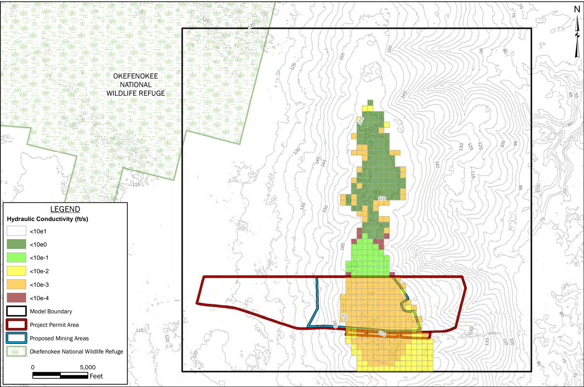
**FIGURE 49: POST-MINING HORIZONTAL HYDRAULIC CONDUCTIVITY LAYER 1**
