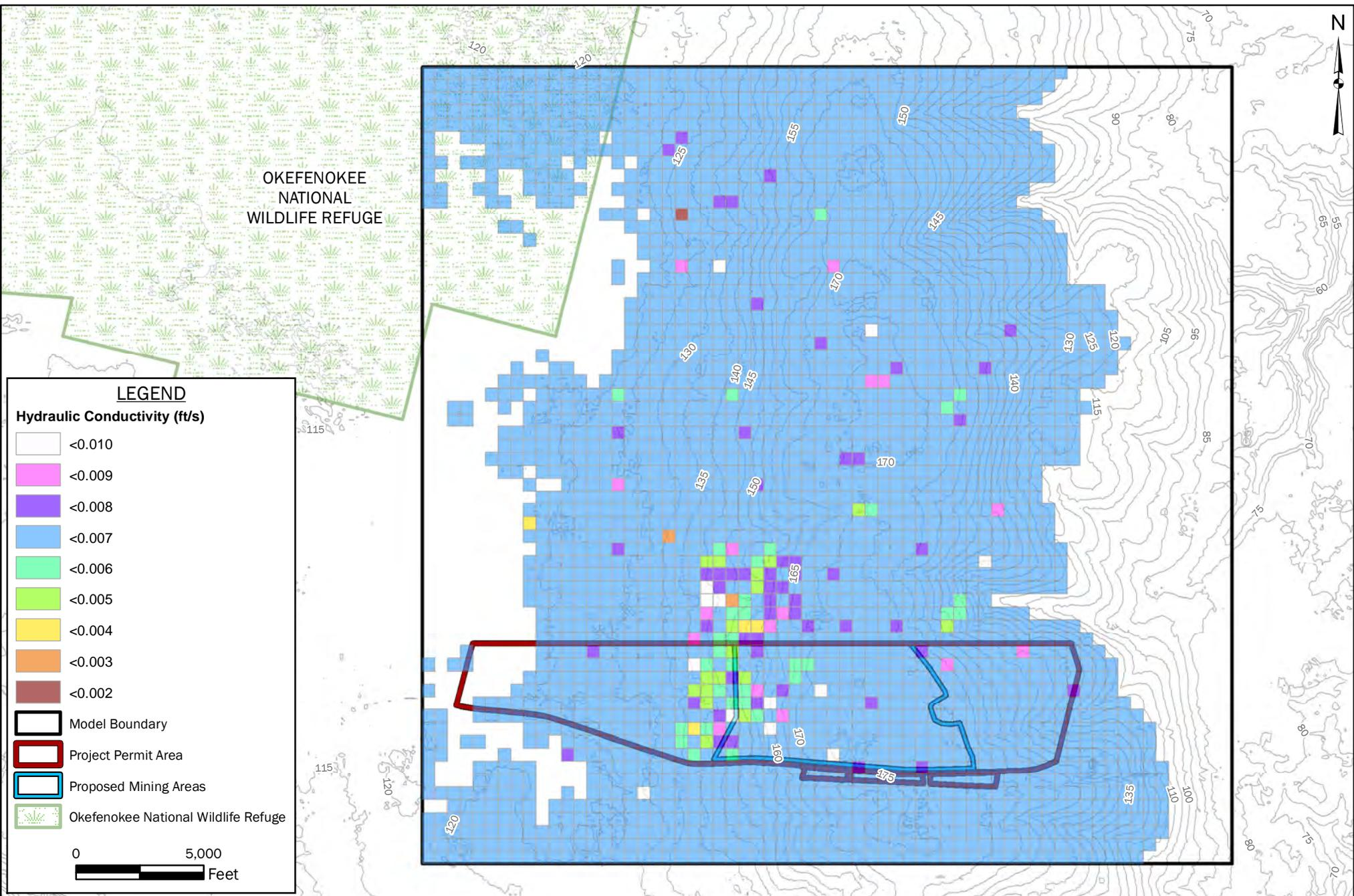
**FIGURE 20: INITIAL MODEL HORIZONTAL HYDRAULIC CONDUCTIVITY LAYER 6**
