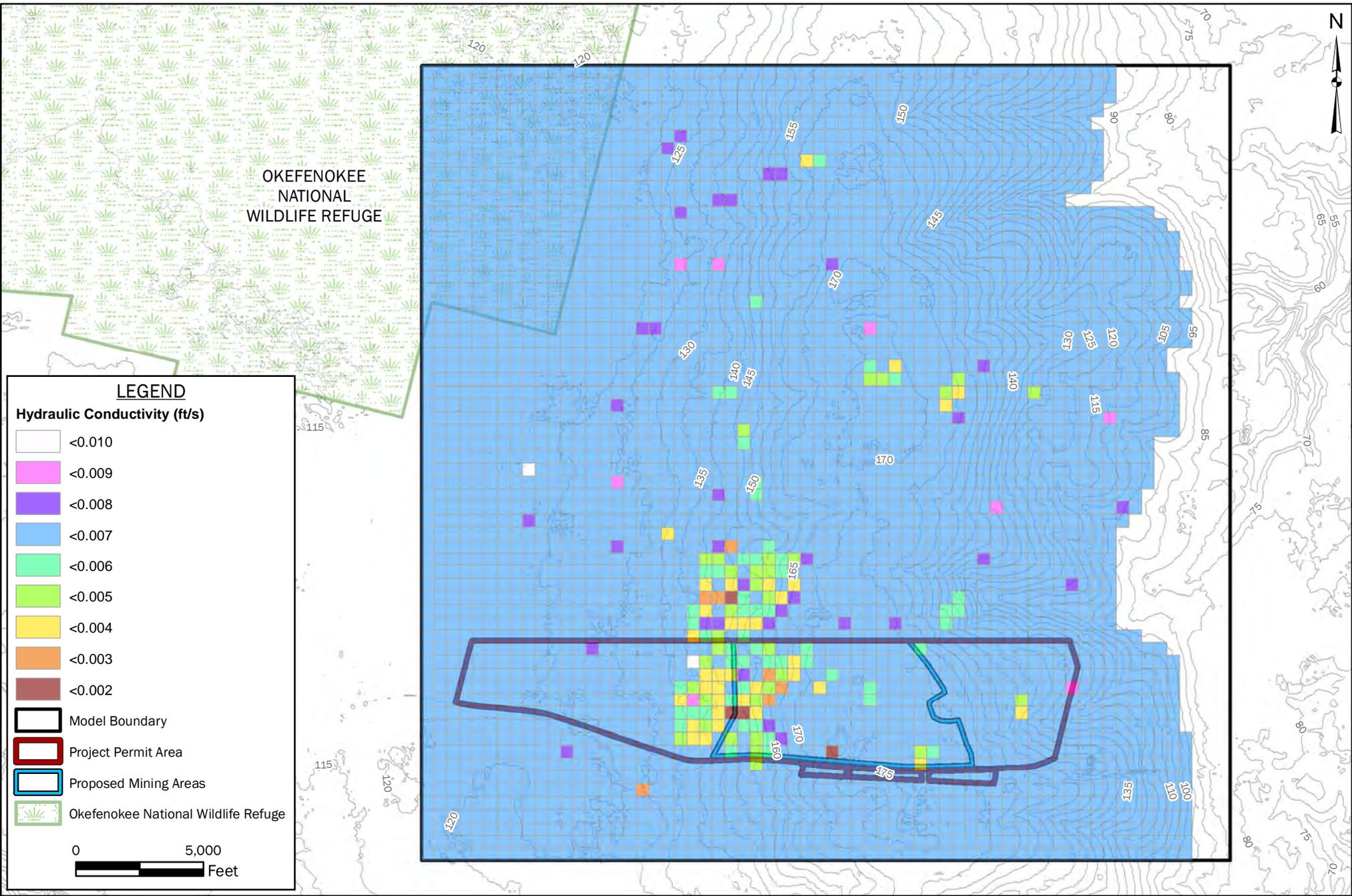
**FIGURE 22: INITIAL MODEL HORIZONTAL HYDRAULIC CONDUCTIVITY LAYER 8**
