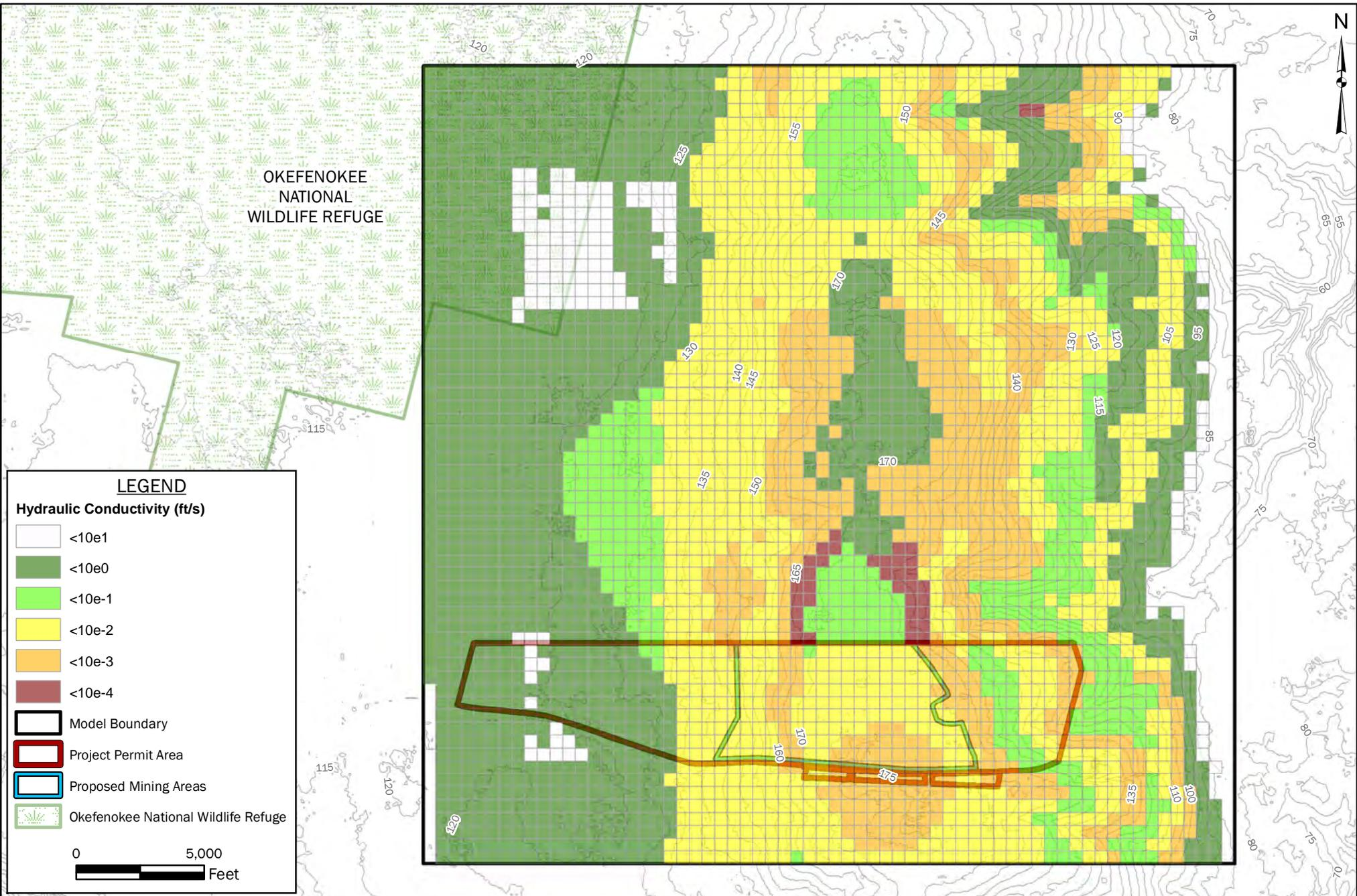
**FIGURE 57: POST-MINING HORIZONTAL HYDRAULIC CONDUCTIVITY LAYER 9**
