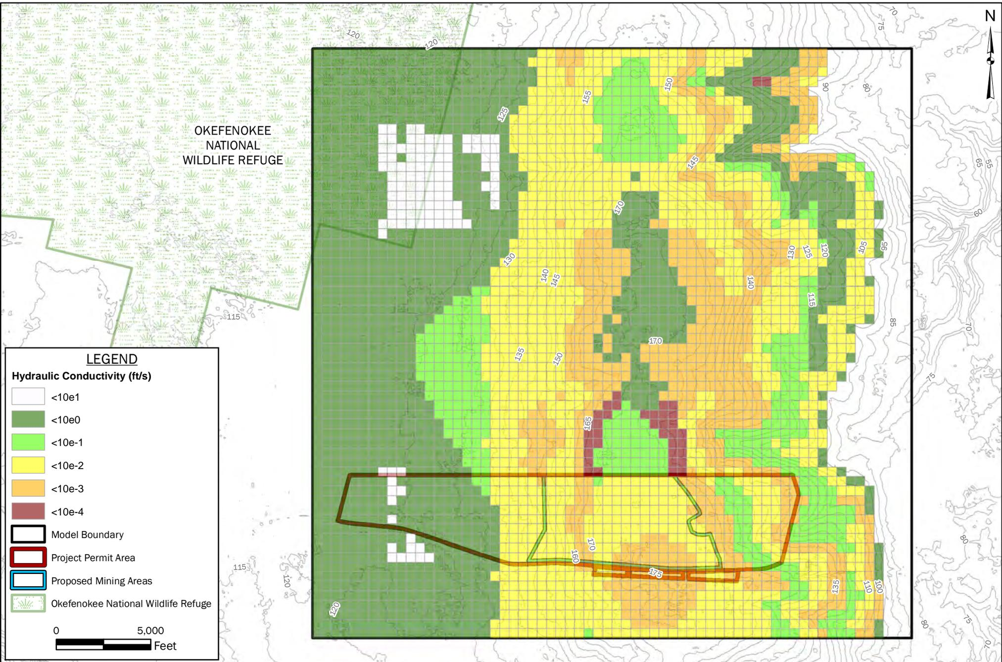
**FIGURE 39: CALIBRATED MODEL HORIZONTAL HYDRAULIC CONDUCTIVITY LAYER 8**
