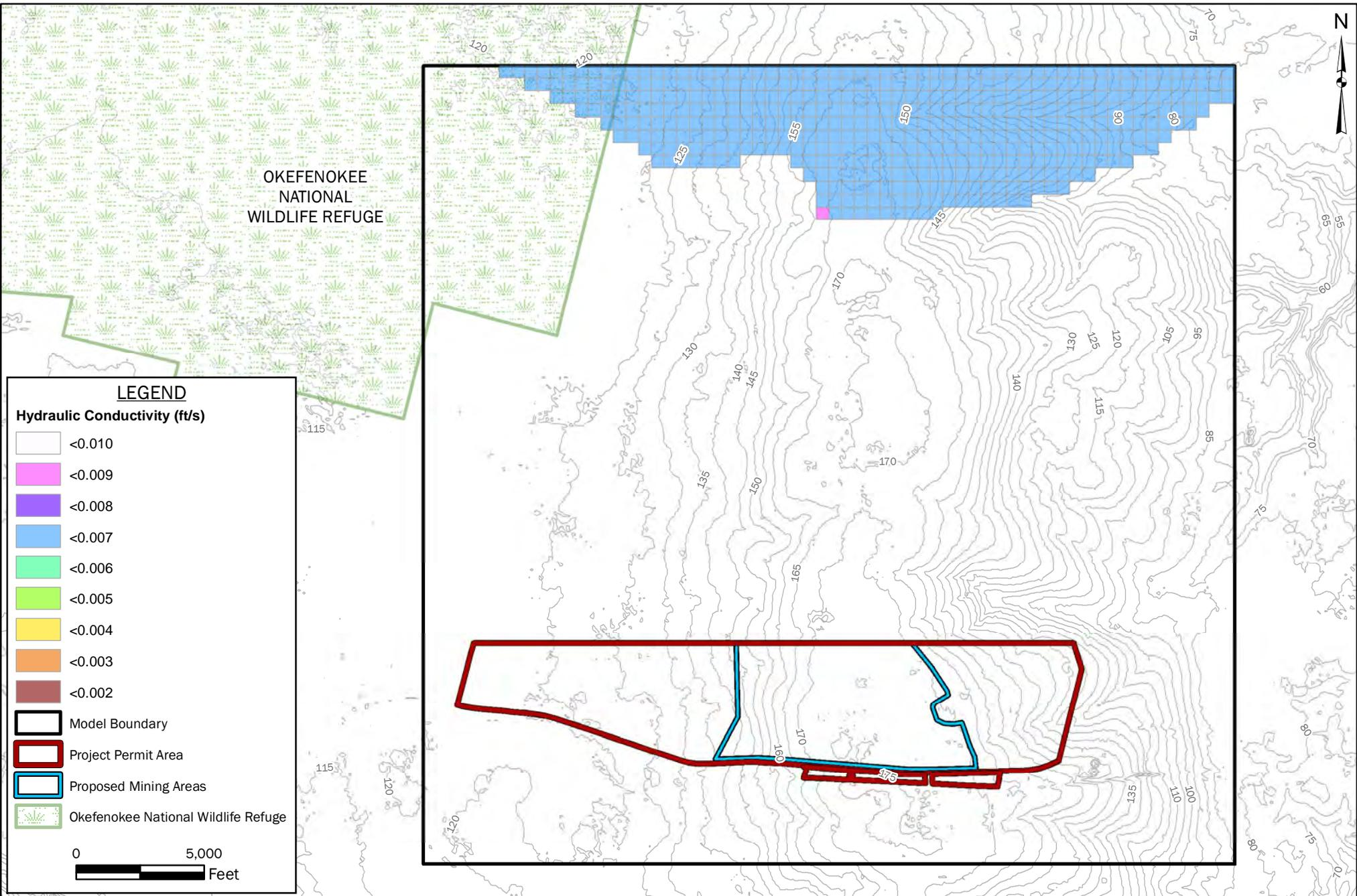
**FIGURE 28: INITIAL MODEL HORIZONTAL HYDRAULIC CONDUCTIVITY LAYER 14**
