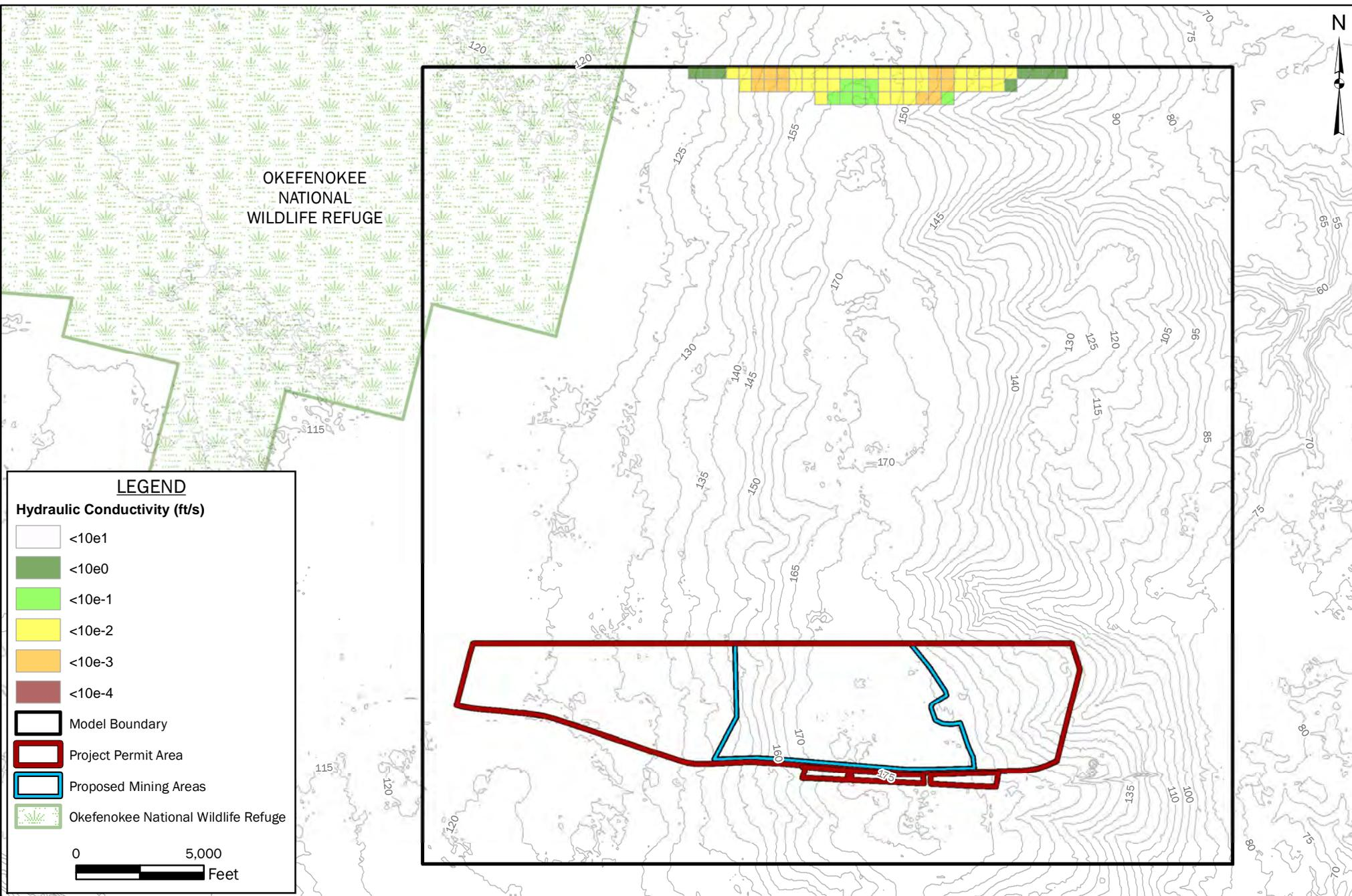
**FIGURE 46: CALIBRATED MODEL HORIZONTAL HYDRAULIC CONDUCTIVITY LAYER 15**
