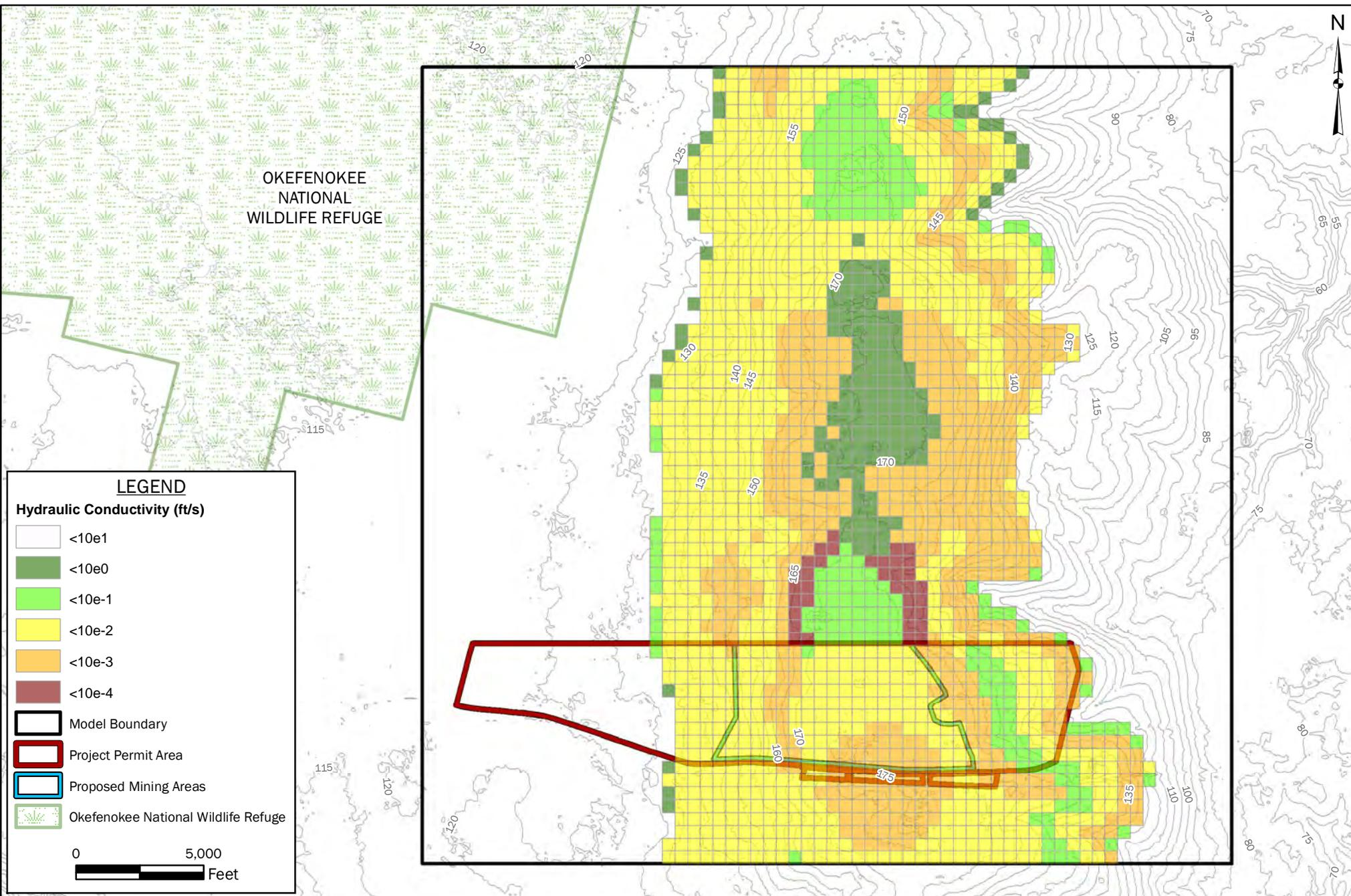
**FIGURE 36: CALIBRATED MODEL HORIZONTAL HYDRAULIC CONDUCTIVITY LAYER 5**
