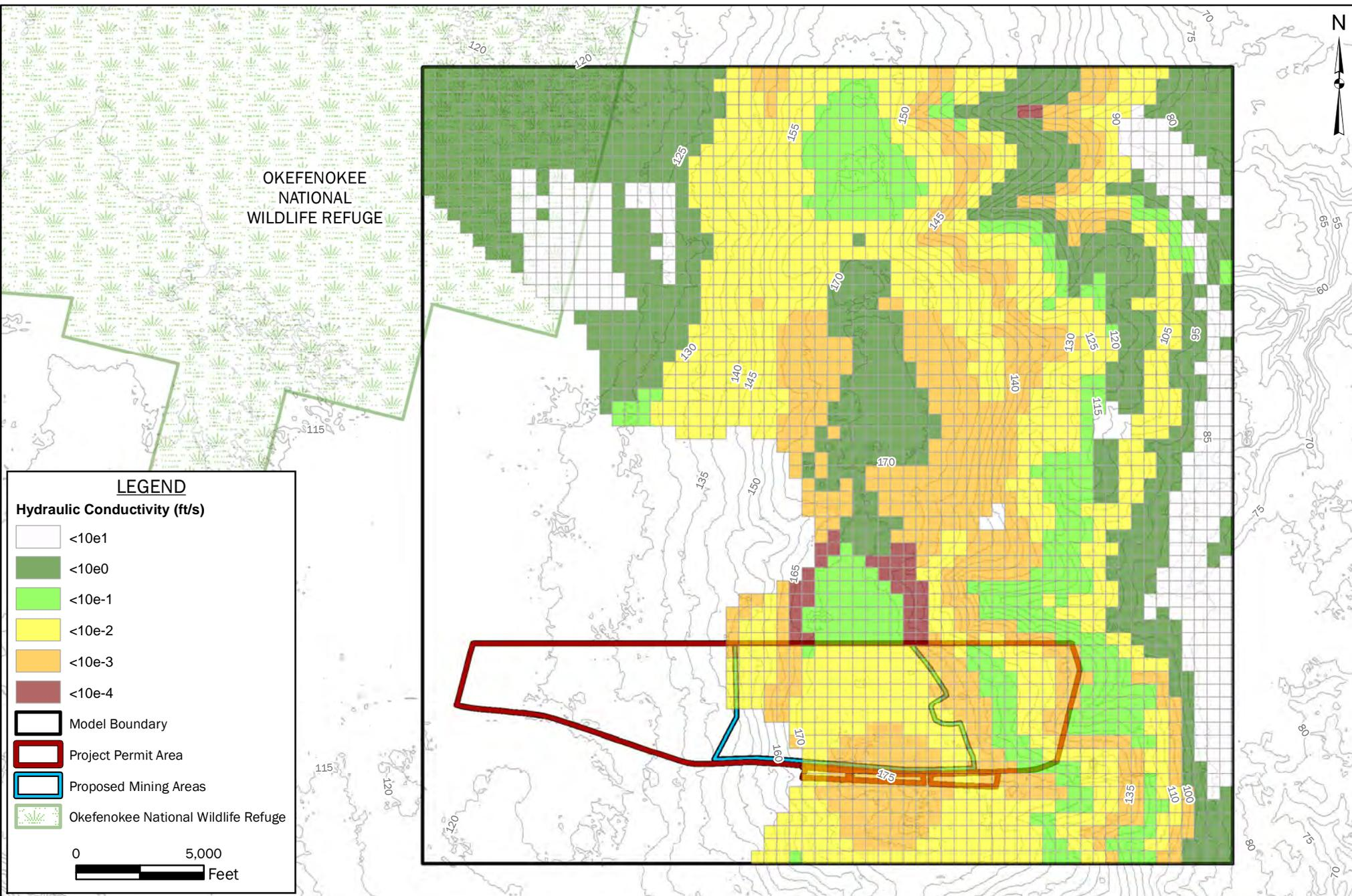
**FIGURE 60: POST-MINING HORIZONTAL HYDRAULIC CONDUCTIVITY
