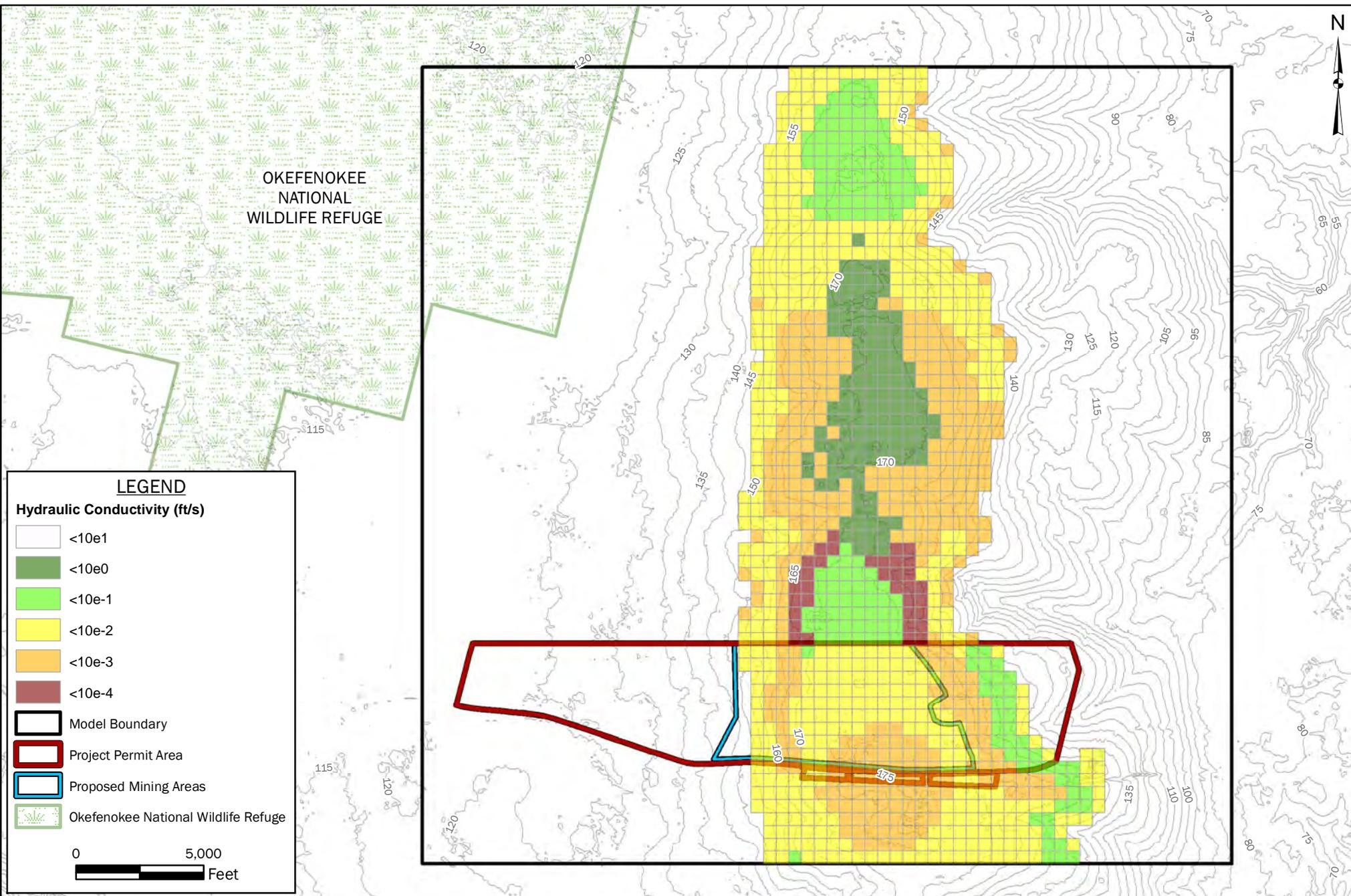
**FIGURE 34: CALIBRATED MODEL HORIZONTAL HYDRAULIC CONDUCTIVITY LAYER 3**
