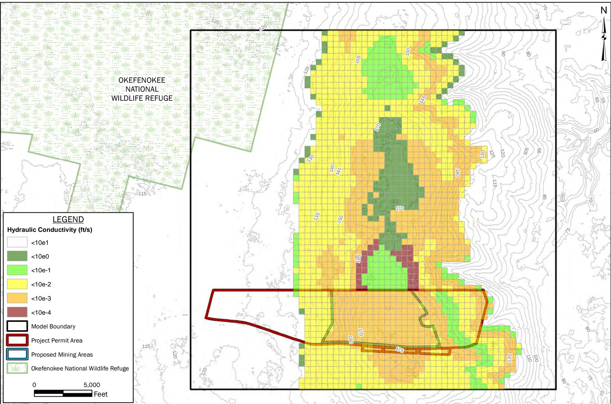
**FIGURE 53: POST-MINING HORIZONTAL HYDRAULIC CONDUCTIVITY
