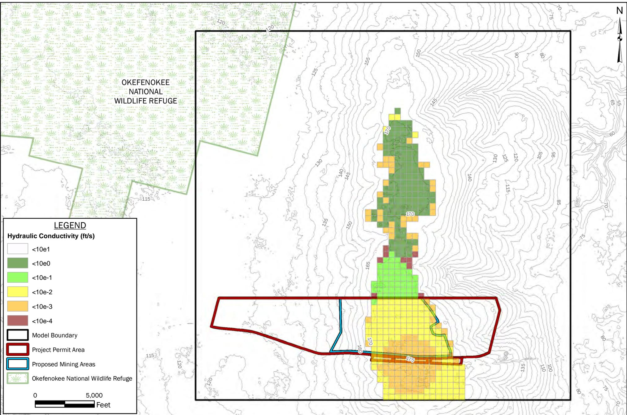
**FIGURE 32: CALIBRATED MODEL HORIZONTAL HYDRAULIC CONDUCTIVITY LAYER 1**
