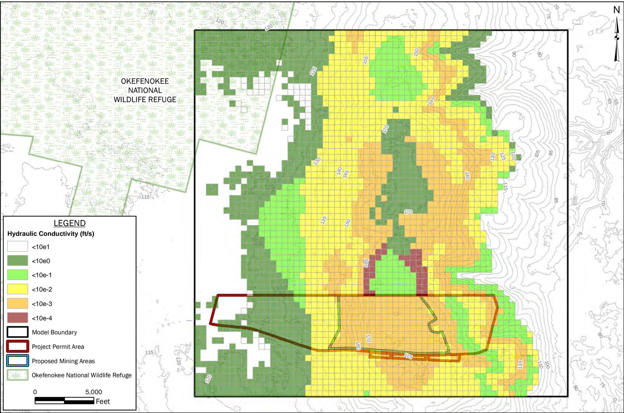
**FIGURE 54: POST-MINING HORIZONTAL HYDRAULIC CONDUCTIVITY LAYER 6**
