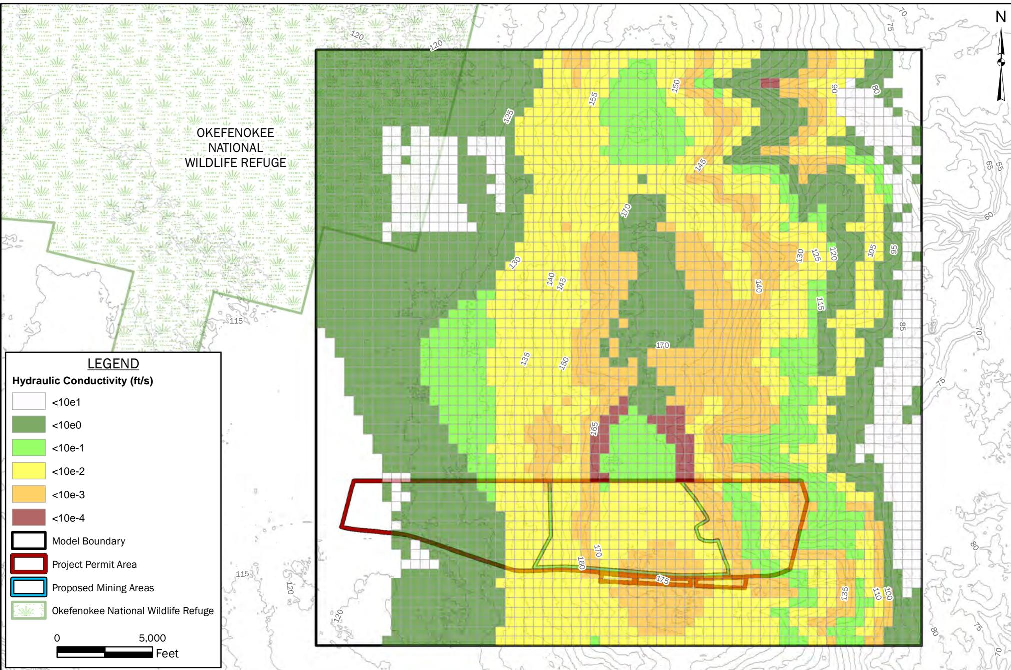
**FIGURE 41: CALIBRATED MODEL HORIZONTAL HYDRAULIC CONDUCTIVITY LAYER 10**
