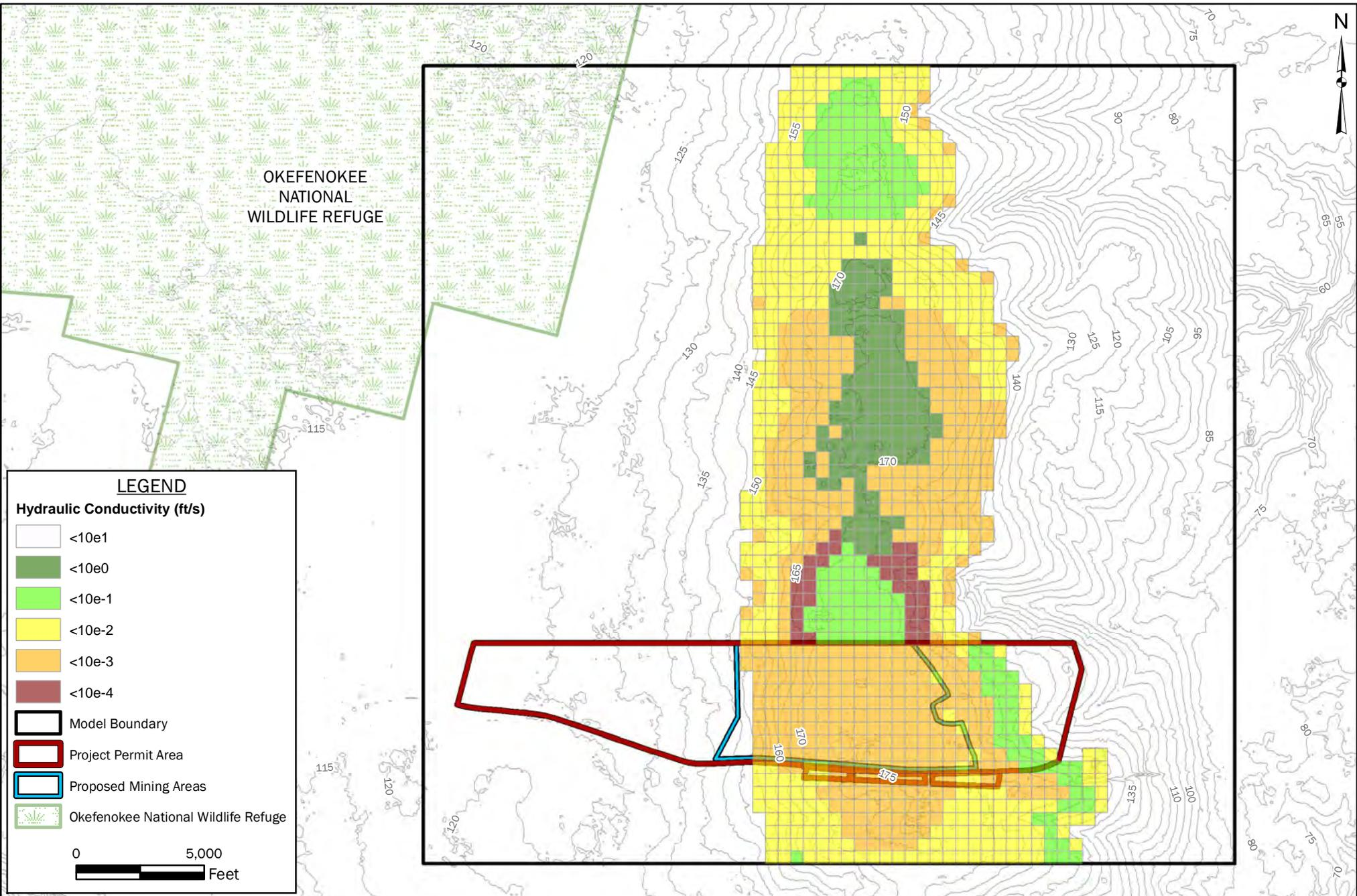
**FIGURE 51: POST-MINING HORIZONTAL HYDRAULIC CONDUCTIVITY
