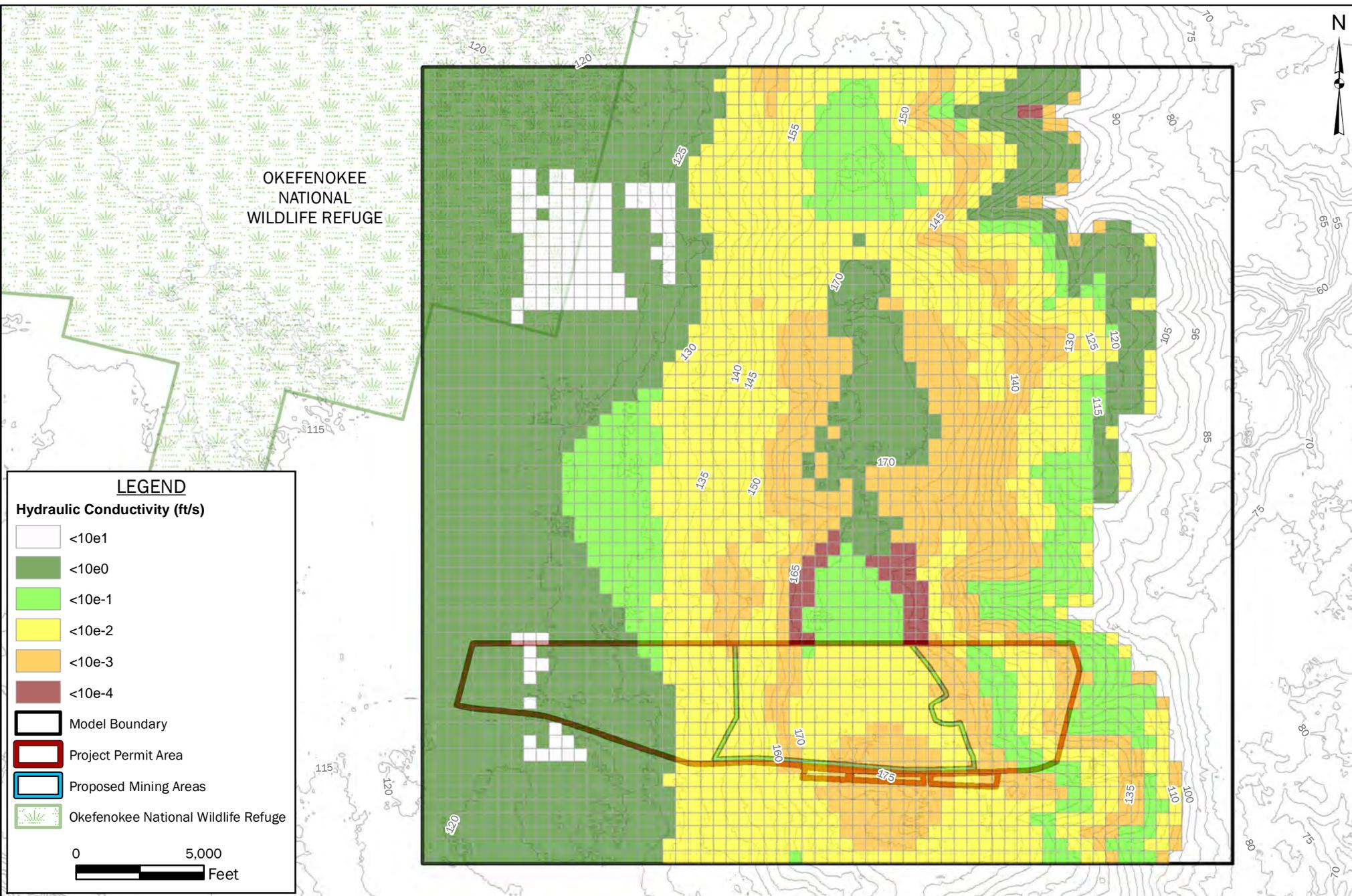
**FIGURE 55: POST-MINING HORIZONTAL HYDRAULIC CONDUCTIVITY
