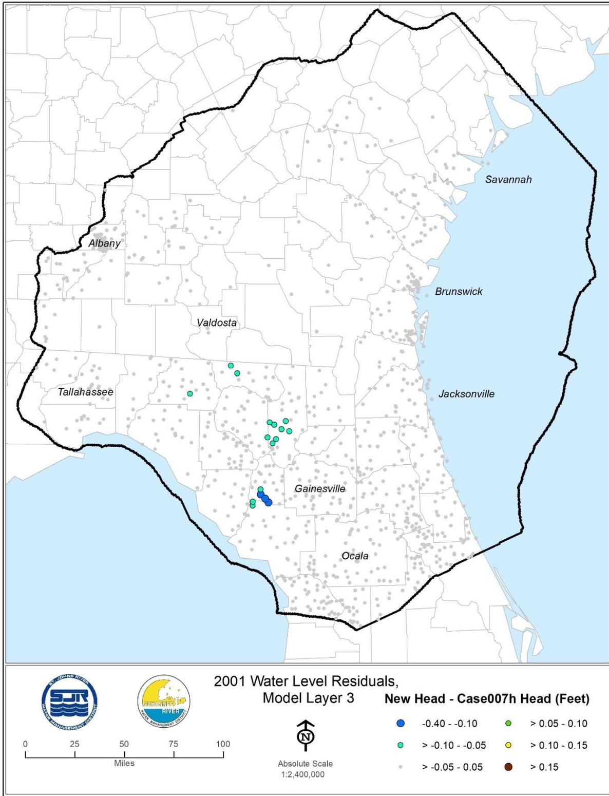
Figure 14. Comparison of groundwater level residuals in Model Layer 3 targets in Suwannee and Columbia County, 2001. The residual was calculated by subtracting the estimated groundwater level from the modelled groundwater level.
