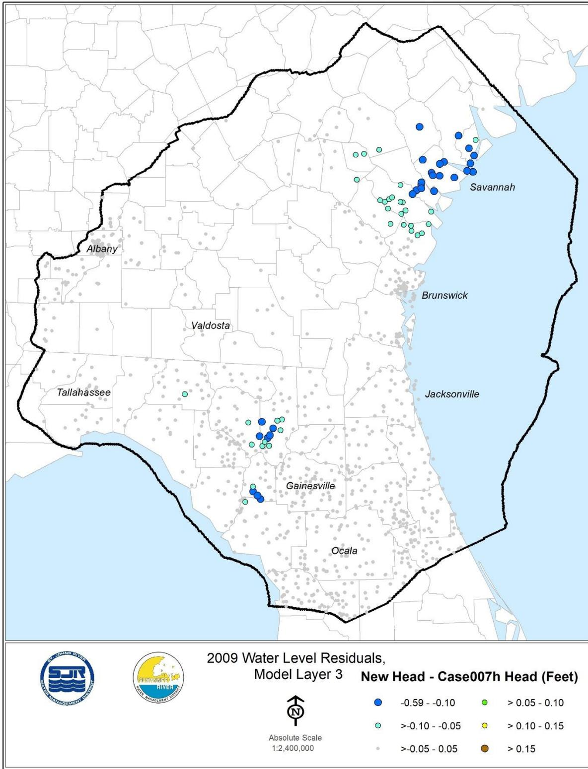
Figure 18. Comparison of groundwater level residuals in Model Layer 3 targets in Suwannee and Columbia County, 2009. The residual was calculated by subtracting the estimated groundwater level from the modelled groundwater level.
