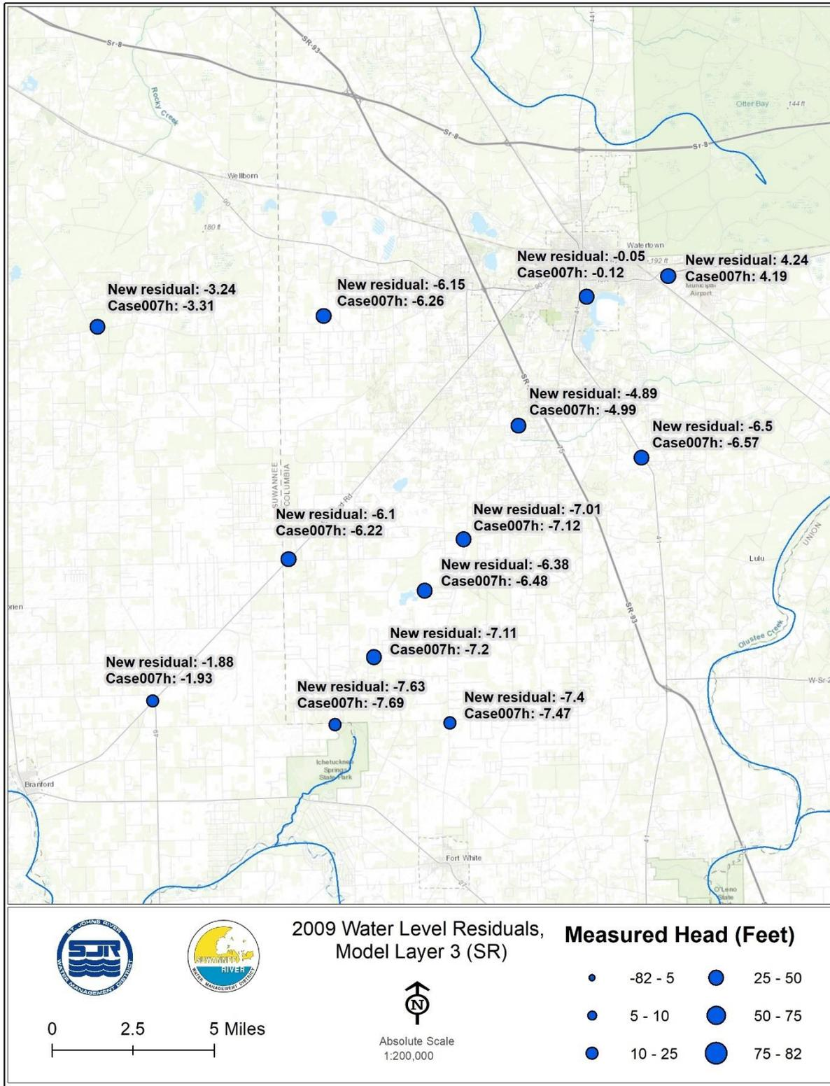
Figure 19. Comparison of groundwater level residuals in Model Layer 3 targets in southern Gilchrist County, 2009. The residual was calculated by subtracting the estimated groundwater level from the modelled groundwater level.
