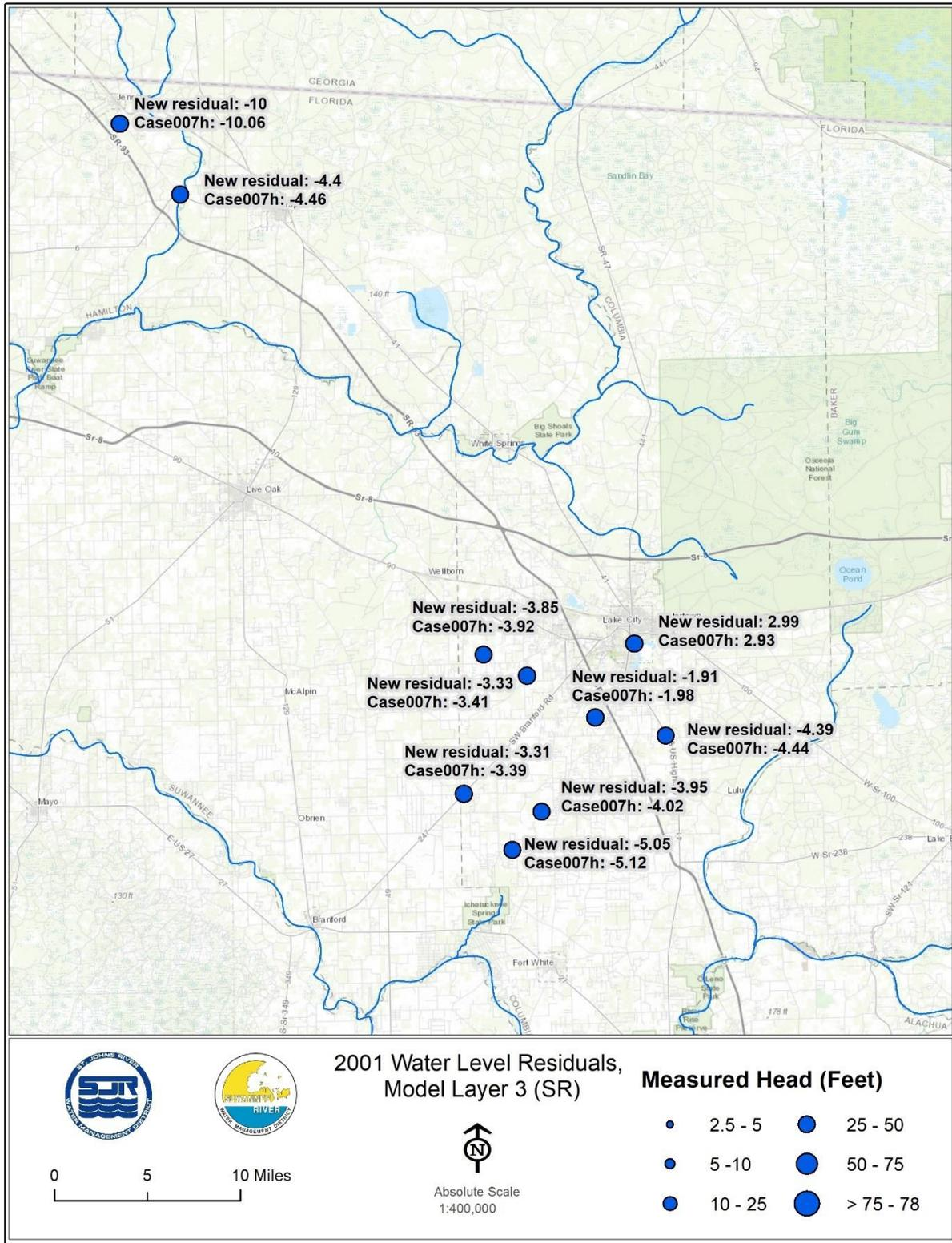
Figure 15. Comparison of groundwater level residuals in Model Layer 3 targets in southern Gilchrist County, 2001. The residual was calculated by subtracting the estimated groundwater level from the modelled groundwater level.
