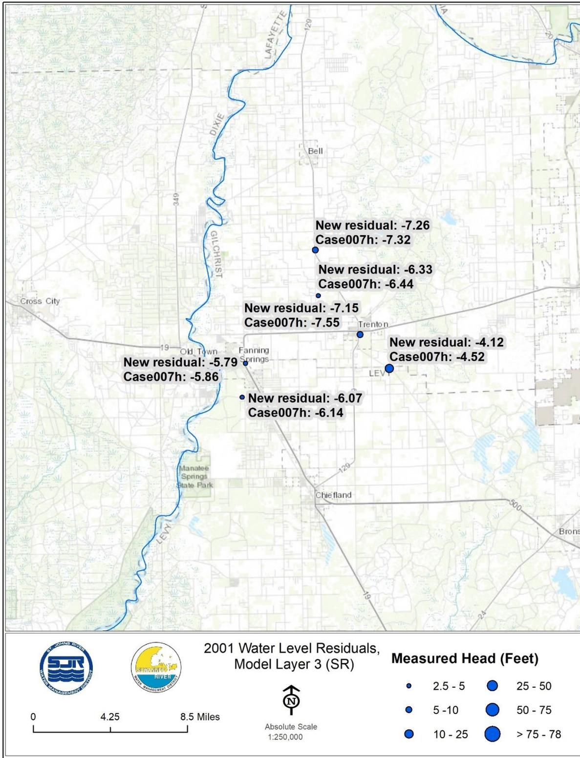
Figure 16. Head difference (in feet) in Model Layer 3, 2001. The head difference was calculated by subtracting the case007h simulated head from the case007h-1 simulated head.
