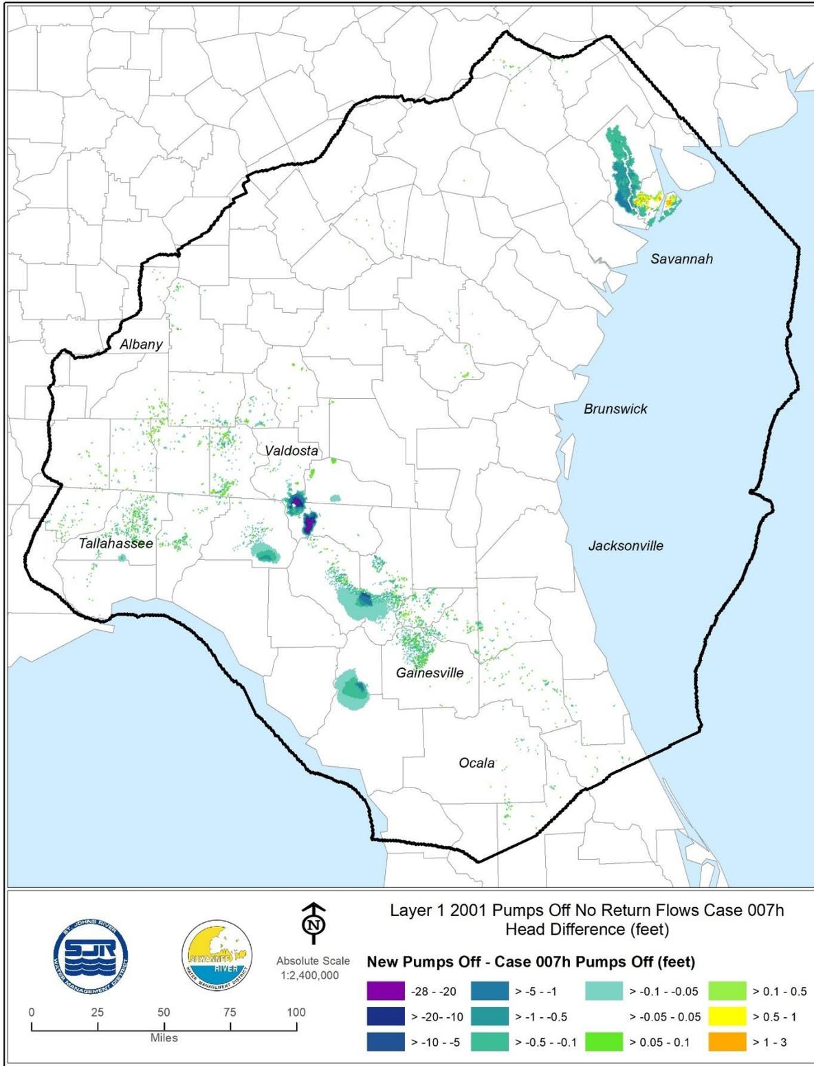
Figure 32. No-pumping head difference (in feet) in Model Layer 1, 2009. The head difference was calculated by subtracting the case007h simulated head from the case007h-1 simulated head.
