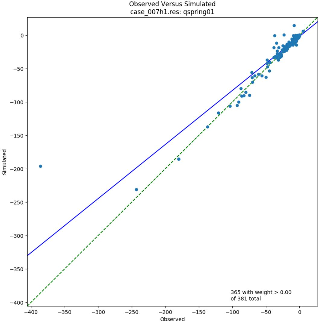
Figure 6. Scatterplot of observed and simulated spring flows for case007h-1, 2009.
