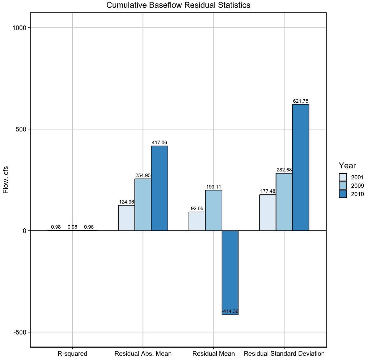
Figure 39. Comparison of case007h-1 baseflow pickup rate residual statistics for 2001, 2009 and 2010.
