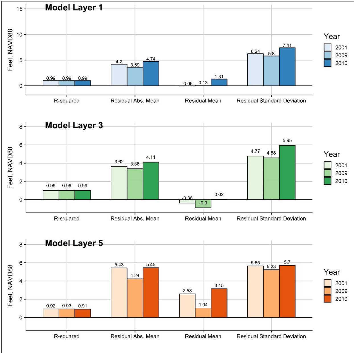
Figure 38. Comparison of case007h-1 cumulative baseflow rate residual statistics for 2001, 2009 and 2010.
