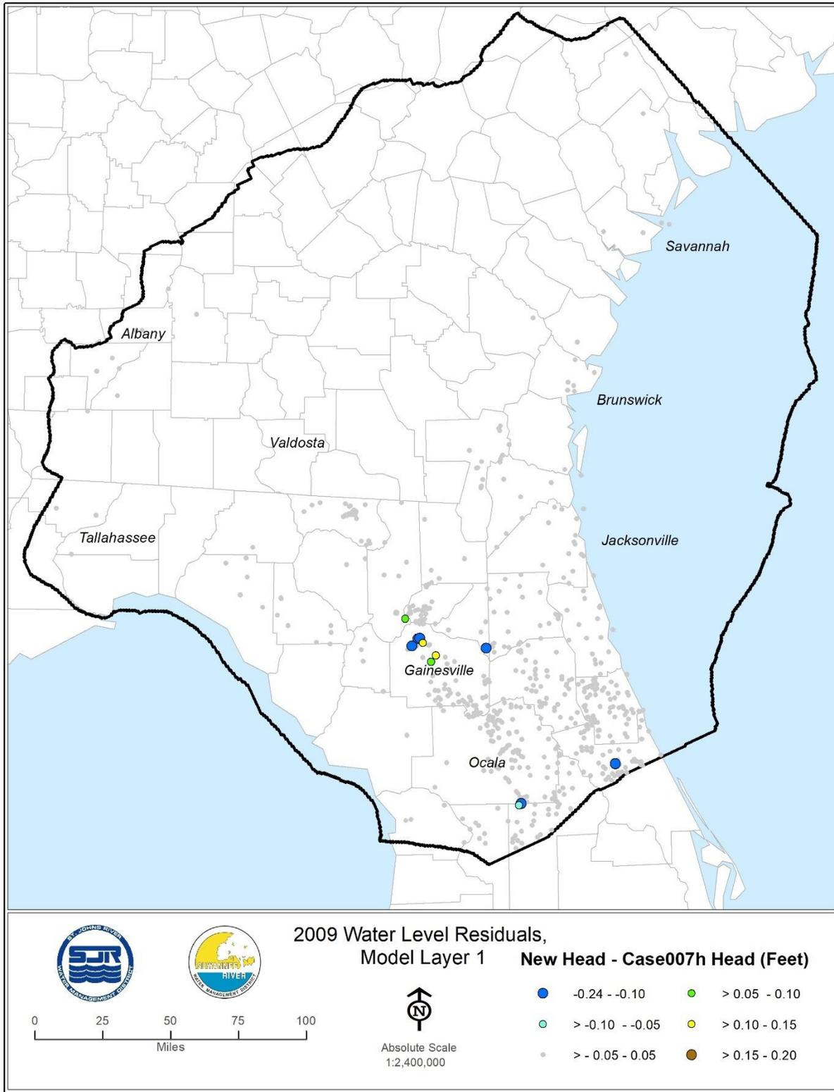
Figure 12. Head difference (in feet) in Model Layer 1, 2009. The head difference was calculated by subtracting the case007h simulated head from the case007h-1 simulated head.
